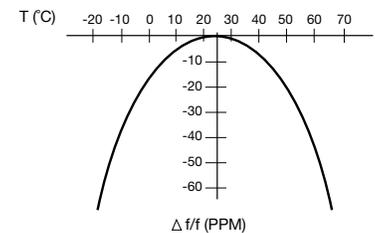
To determine frequency stability, use parabolic curvature. For example: What is the stability at 45°C?
