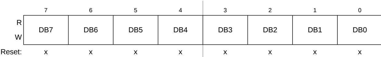
Figure 11-34. Data Segment Registers (DSR0–DSR7) — Extended Identifier Mapping
