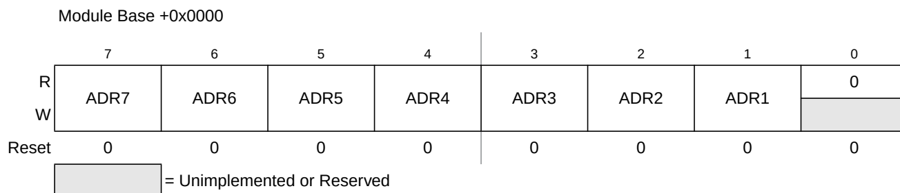
Figure 12-3. IIC Bus Address Register (IBAD)
