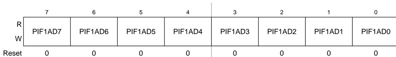
Figure 2-75. Port F Interrupt Flag Register (PIF1AD)
