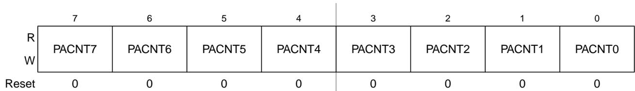
**Figure 16-27. Pulse Accumulator Count Register Low (PACNTL)**
