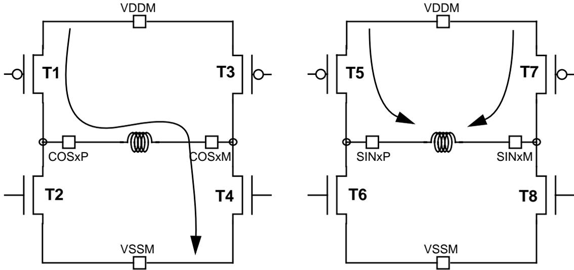
**Figure 21-11. Current Flow when STEP = 0, DCOIL = 1, ITG = 0, RCIR = 0**
