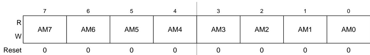
**Figure 11-23. MSCAN Identifier Mask Registers (Second Bank) — CANIDMR4–CANIDMR7**
