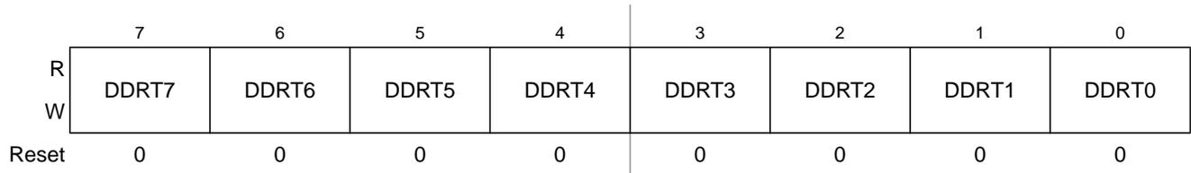
**Figure 2-14. Port T Data Direction Register (DDRT)**
