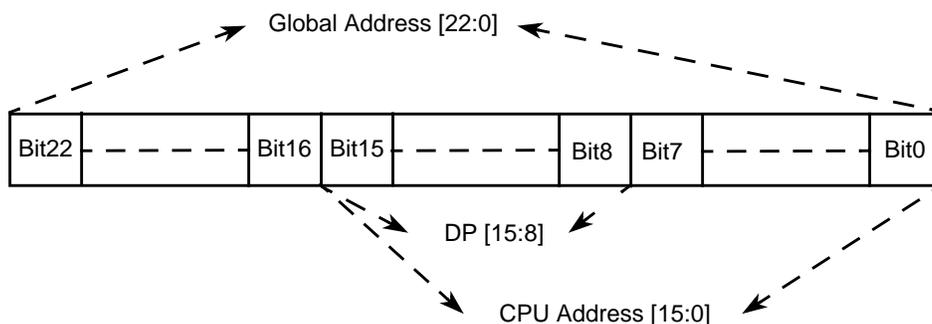
Figure 3-9. DIRECT Address Mapping
