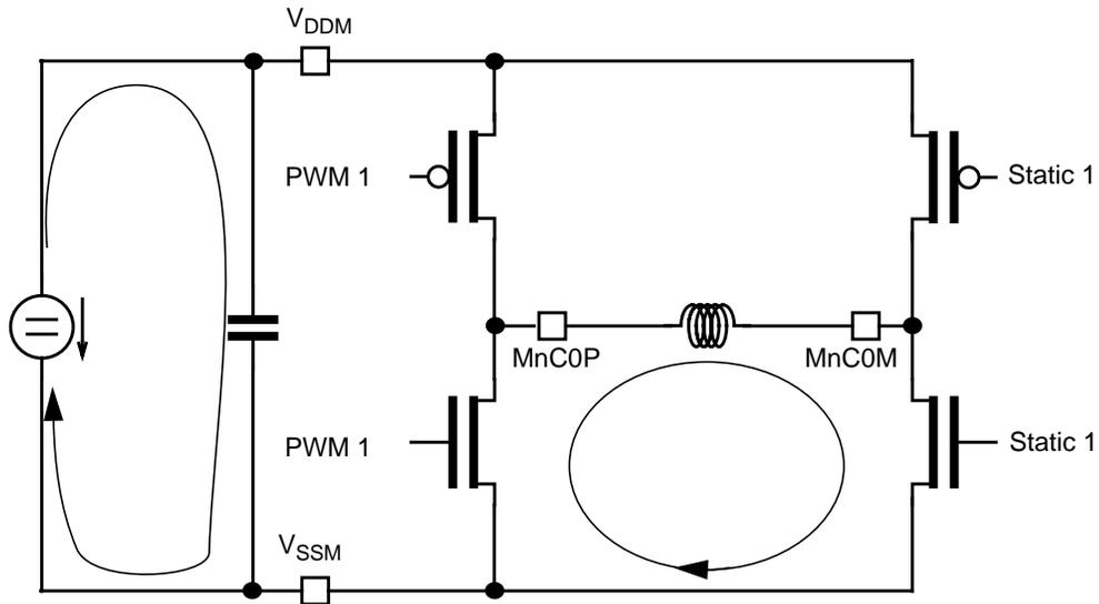
Figure 20-15. PWM Passive Phase, RECIRC = 1, S = 0
