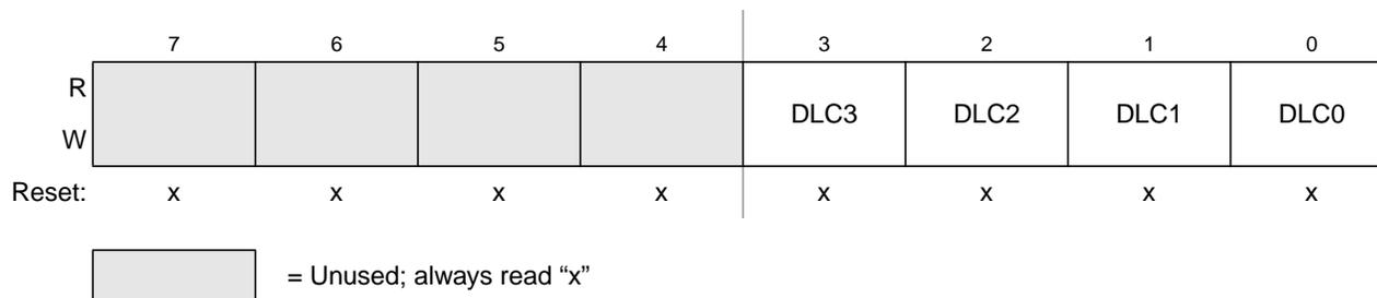
Figure 11-35. Data Length Register (DLR) — Extended Identifier Mapping
