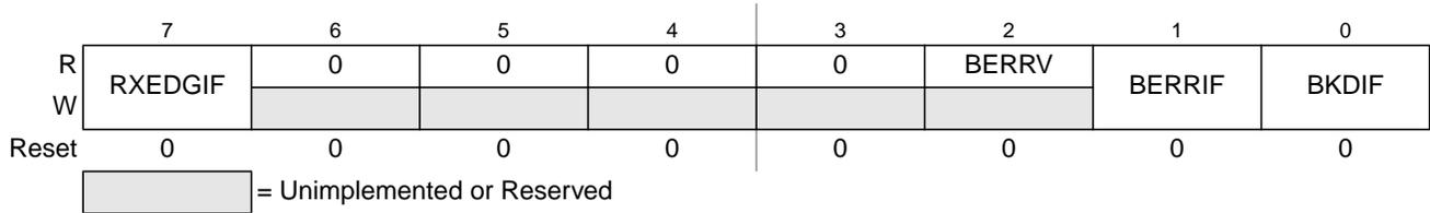
**Figure 14-6. SCI Alternative Status Register 1 (SCIASR1)**
