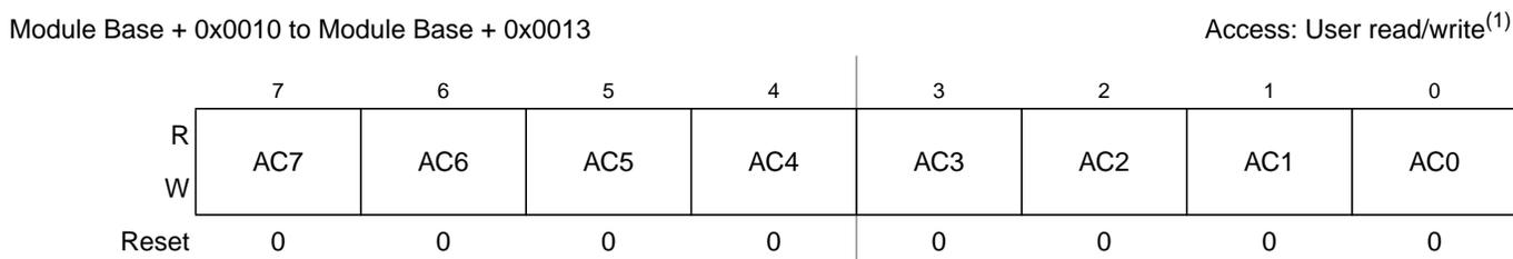
**Figure 11-20. MSCAN Identifier Acceptance Registers (First Bank) — CANIDAR0–CANIDAR3**
