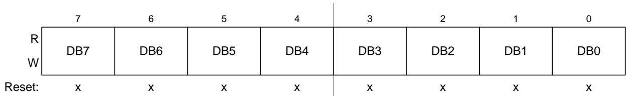
**Figure 11-34. Data Segment Registers (DSR0–DSR7) — Extended Identifier Mapping**
