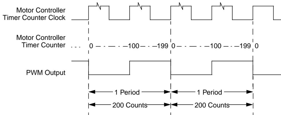
**Figure 20-17. PWM Output: DITH = 0, MCAM[1:0] = 01, MCDC = 100, MCPER = 200, RECIRC = 0**
