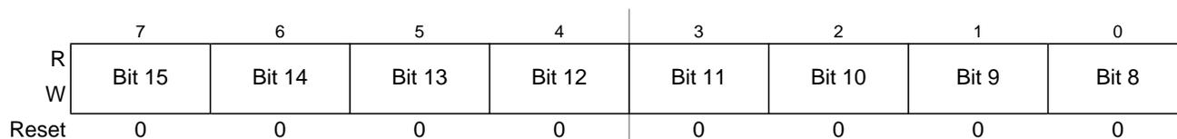
Figure 6-18. Debug Comparator Data High Register (DBGXDH)
