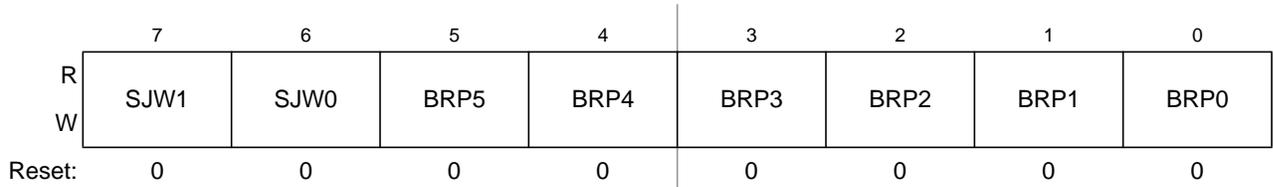
**Figure 11-6. MSCAN Bus Timing Register 0 (CANBTR0)**
