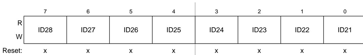
Figure 11-26. Identifier Register 0 (IDR0) — Extended Identifier Mapping
