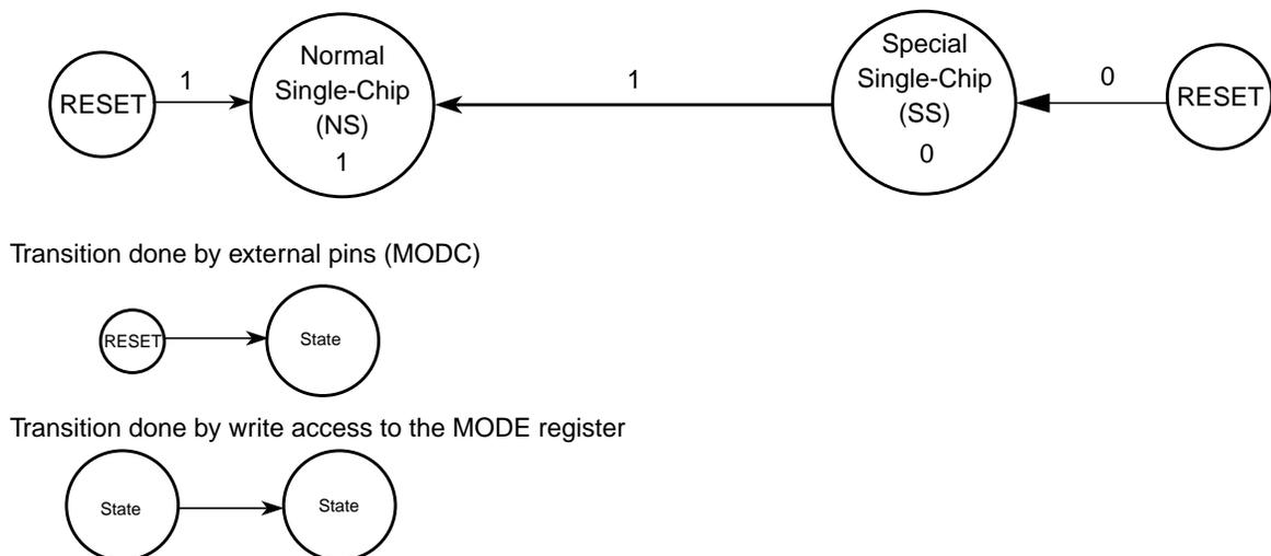
**Figure 3-5. Mode Transition Diagram when MCU is Unsecured**
