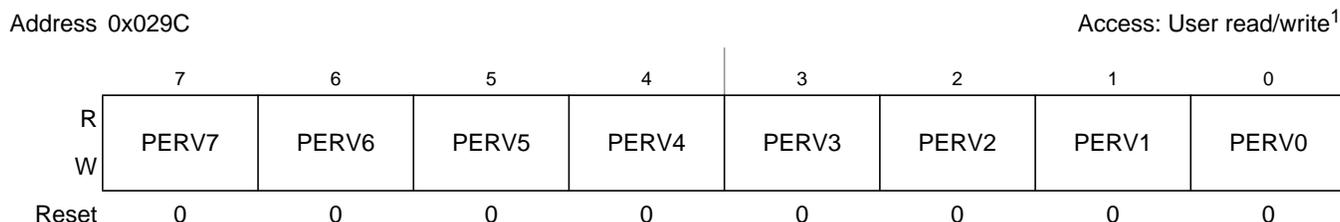
**Figure 2-90. Port V Pull Device Enable Register (PERV)**
