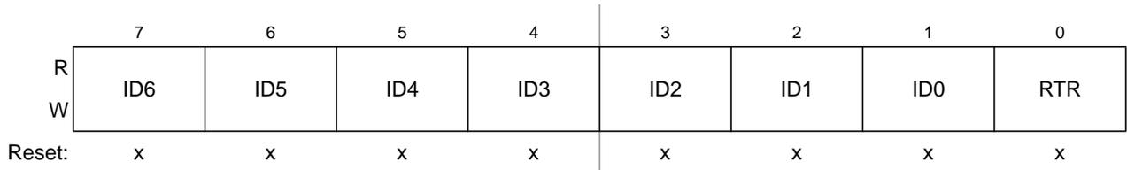
**Figure 11-29. Identifier Register 3 (IDR3) — Extended Identifier Mapping**
