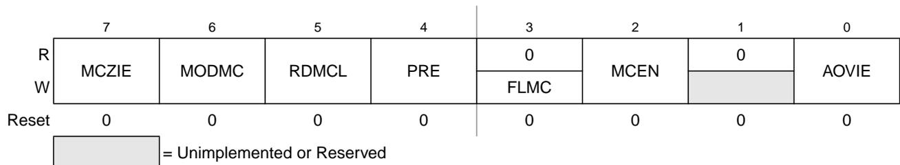
**Figure 21-3. Modulus Down Counter Control Register (MDCCTL)**
