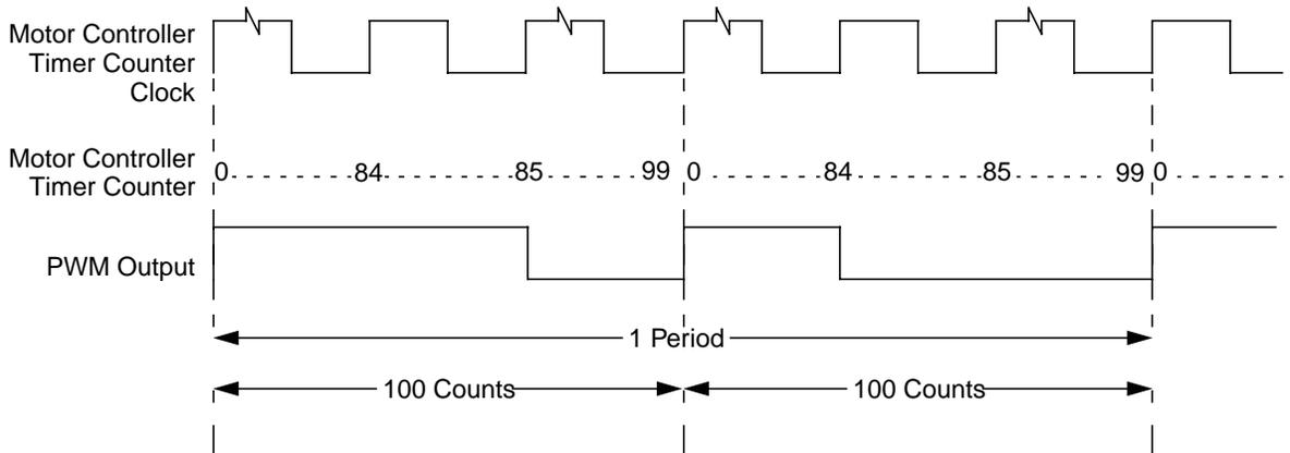
**Figure 20-20. PWM Output: DITH = 1, MCAM[1:0] = 10, MCDC = 31, MCPER = 200, RECIRC = 0**
