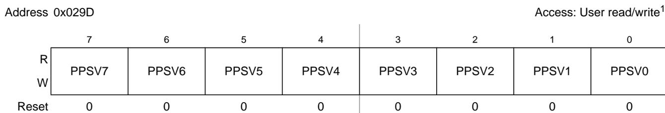
**Figure 2-91. Port V Polarity Select Register (PPSV)**
