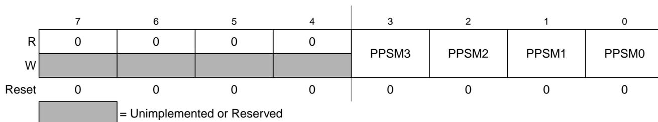
**Figure 2-33. Port M Polarity Select Register (PPSM)**
