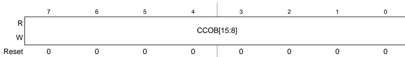
**Figure 18-16. Flash Common Command Object High Register (FCCOBHI)**
