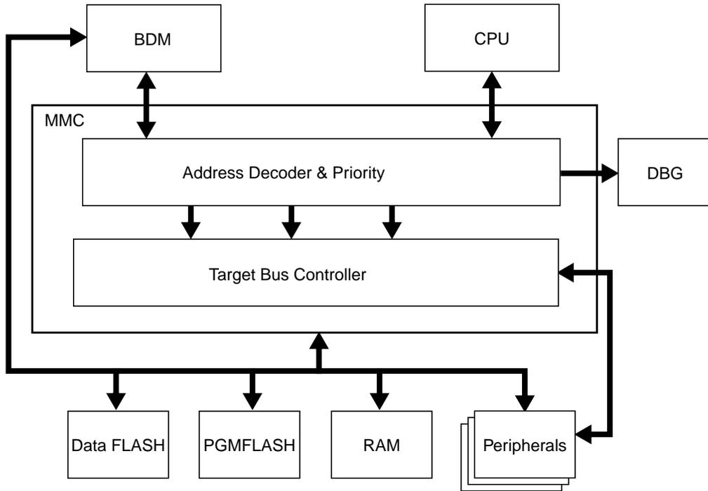
Figure 3-1. MMC Block Diagram
