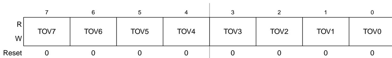
**Figure 16-13. Timer Toggle On Overflow Register 1 (TTOV)**
