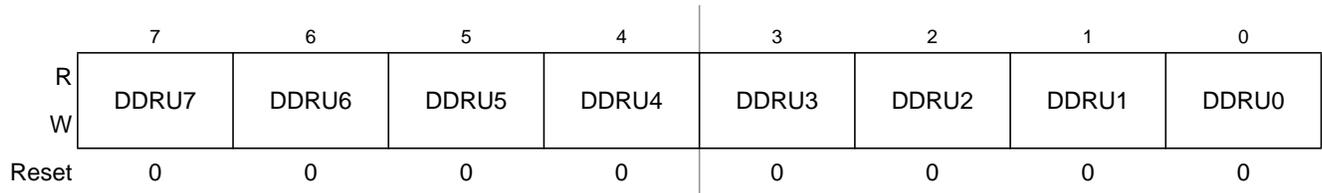
**Figure 2-80. Port U Data Direction Register (DDRU)**
