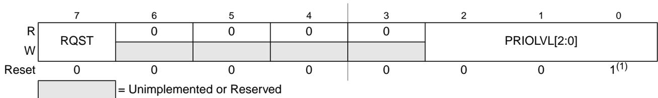
**Figure 4-13. Interrupt Request Configuration Data Register 7 (INT\_CFDATA7)**
