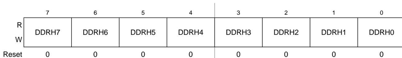
**Figure 2-46. Port H Data Direction Register (DDRH)**
