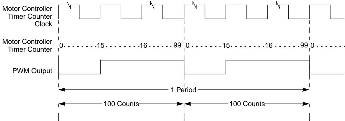
**Figure 20-19. PWM Output: DITH = 1, MCAM[1:0] = 01, MCDC = 30, MCPER = 200, RECIRC = 0**
