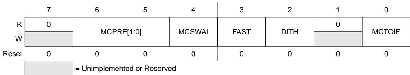
Figure 20-3. Motor Controller Control Register 0 (MCCTL0)
