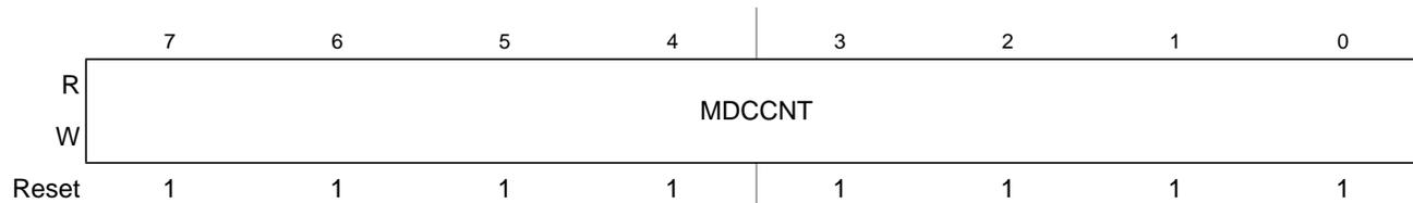
Figure 21-7. Modulus Down-Counter Count Register Low (MDCCNT)
