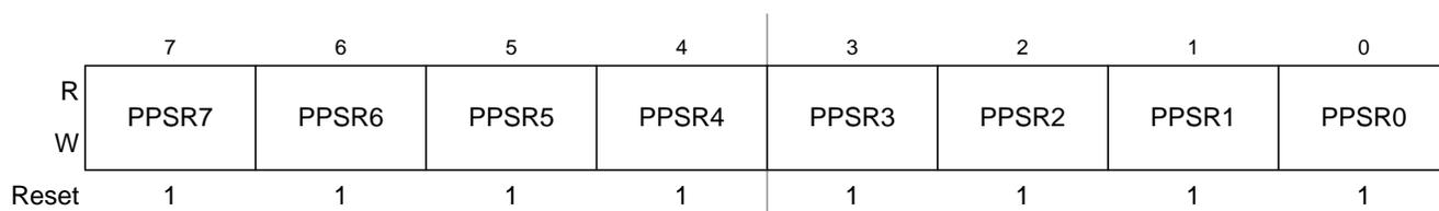
**Figure 2-67. Port R Polarity Select Register (PPSR)**
