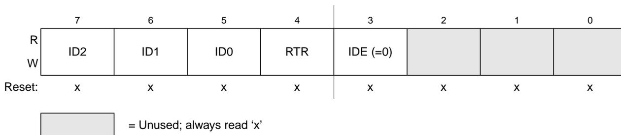
Figure 11-31. Identifier Register 1 — Standard Mapping
