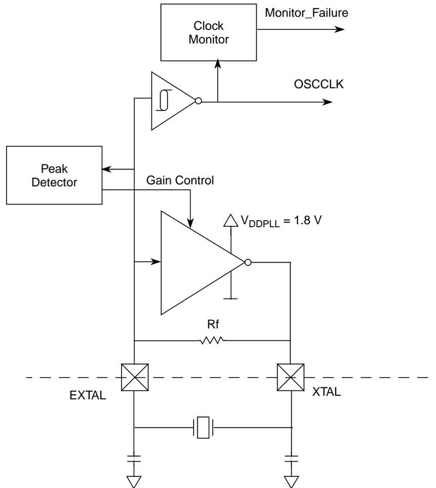
Figure 8-1. XOSC Block Diagram
