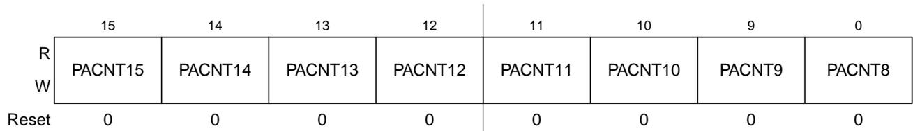
**Figure 16-26. Pulse Accumulator Count Register High (PACNTH)**
