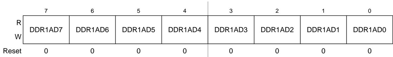
**Figure 2-56. Port AD Data Direction Register (DDR1AD)**
