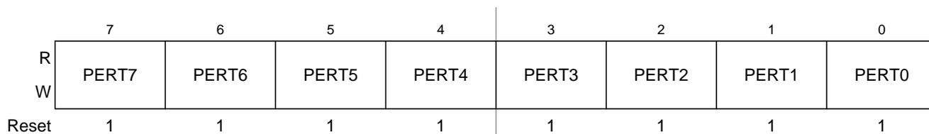
Figure 2-16. Port T Pull Device Enable Register (PERT)
