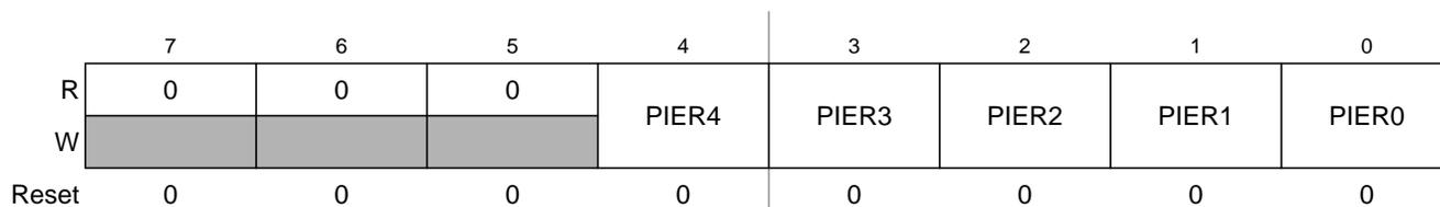
Figure 2-76. Port R Interrupt Enable Register (PIER)
