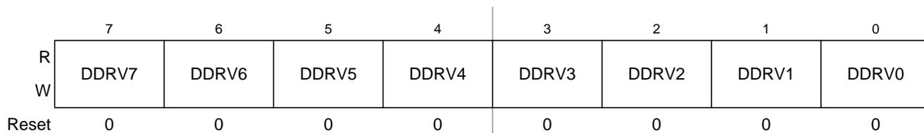
**Figure 2-88. Port V Data Direction Register (DDRV)**
