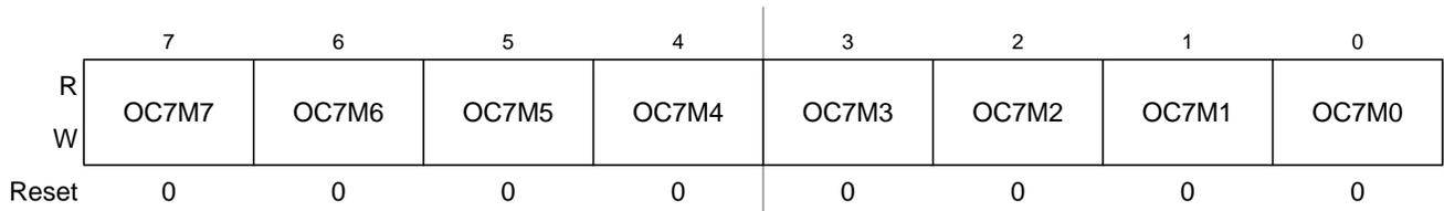
**Figure 16-8. Output Compare 7 Mask Register (OC7M)**
