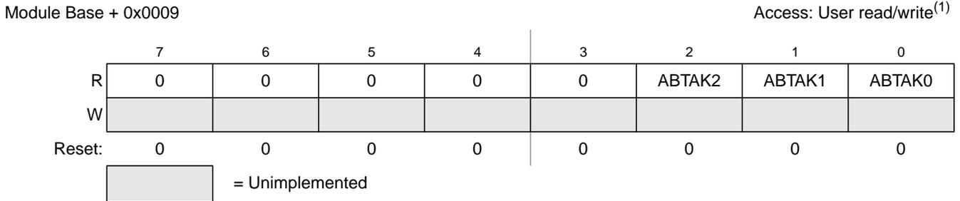
**Figure 11-13. MSCAN Transmitter Message Abort Acknowledge Register (CANTAACK)**
