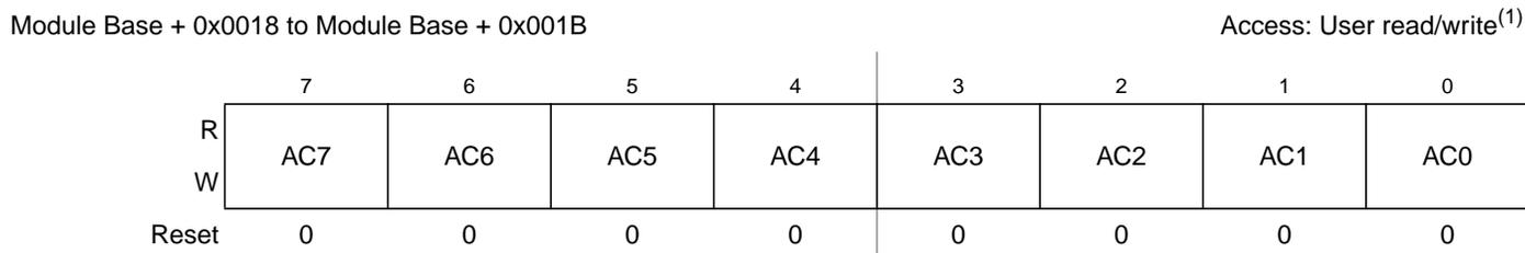
**Figure 11-21. MSCAN Identifier Acceptance Registers (Second Bank) — CANIDAR4–CANIDAR7**
