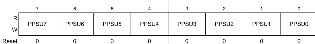
Figure 2-83. Port U Polarity Select Register (PPSU)
