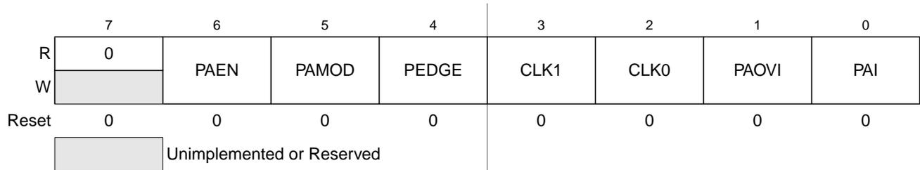
**Figure 16-24. 16-Bit Pulse Accumulator Control Register (PACTL)**
