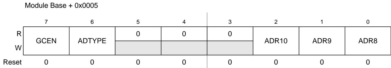
Figure 12-9. IIC Bus Control Register 2(BCR2)
