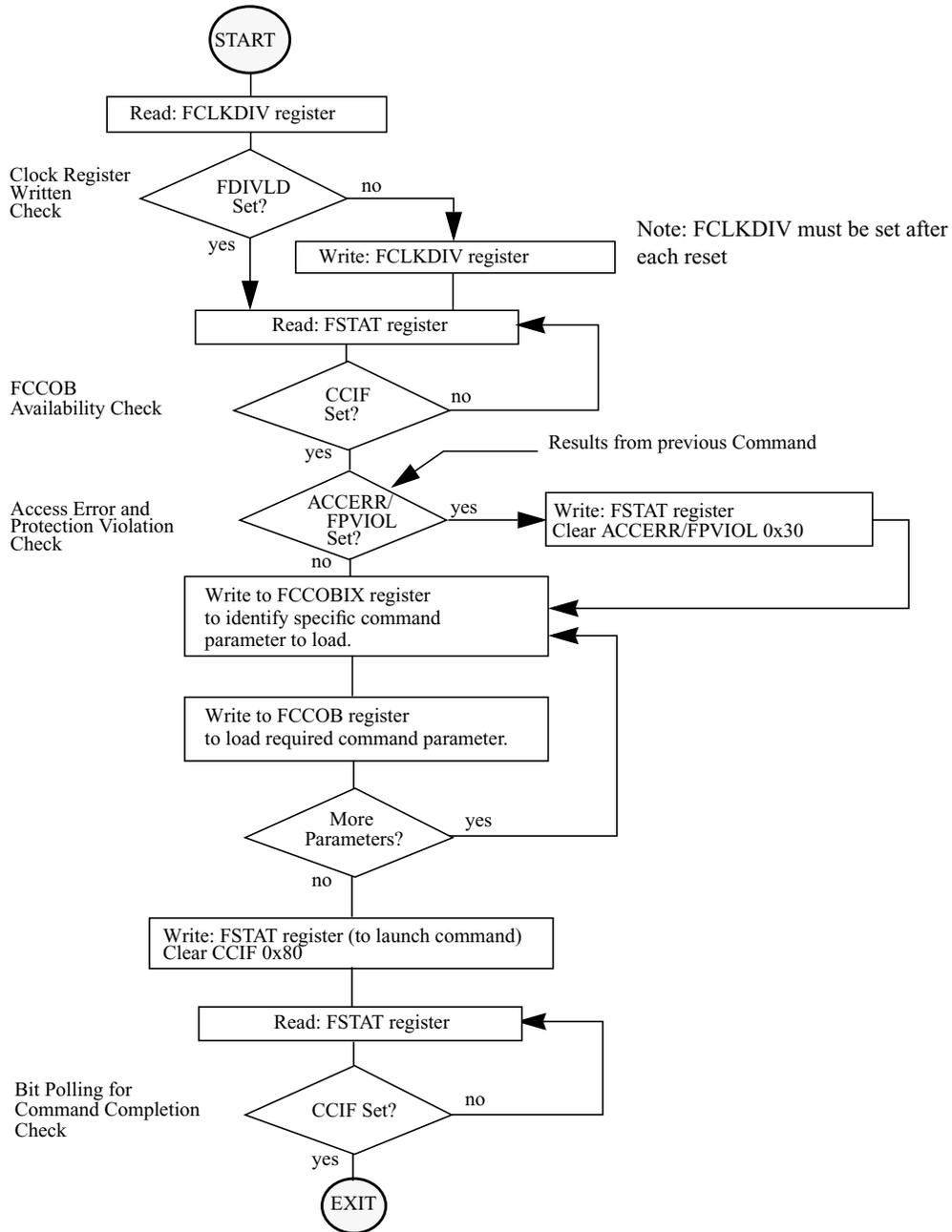
Figure 18-26. Generic Flash Command Write Sequence Flowchart
