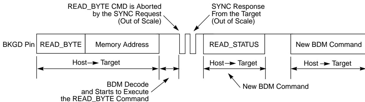
**Figure 5-13. ACK Abort Procedure at the Command Level**
