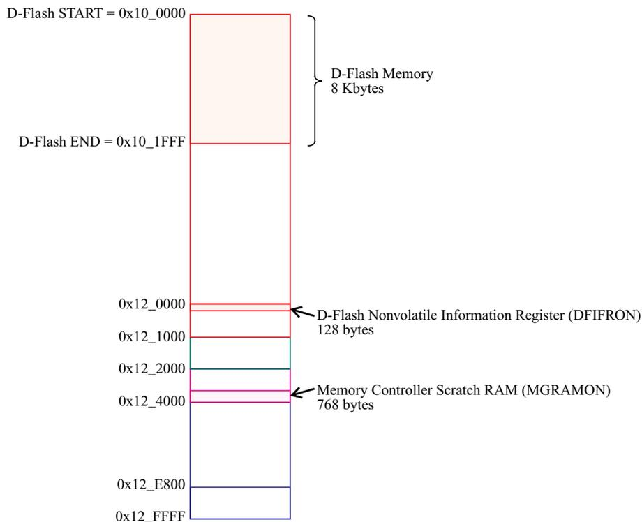
Figure 19-3. D-Flash and Memory Controller Resource Memory Map
