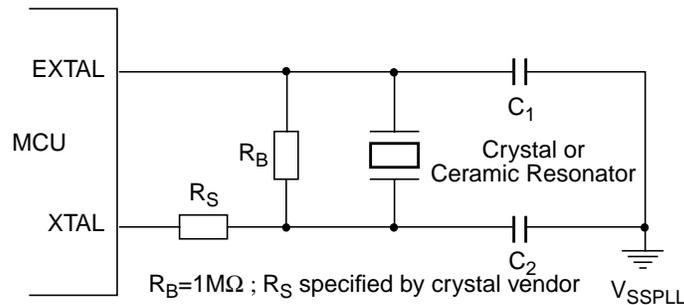
**Figure 1-7. Full Swing Pierce Oscillator Connections (XCLKS = 1)**
