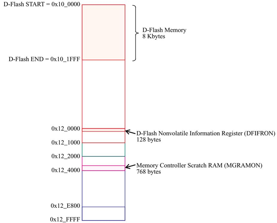
Figure 18-3. D-Flash and Memory Controller Resource Memory Map
