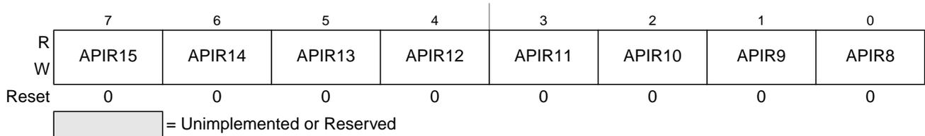
**Figure 9-5. Autonomous Periodical Interrupt Rate High Register (VREGAPIRH)**
