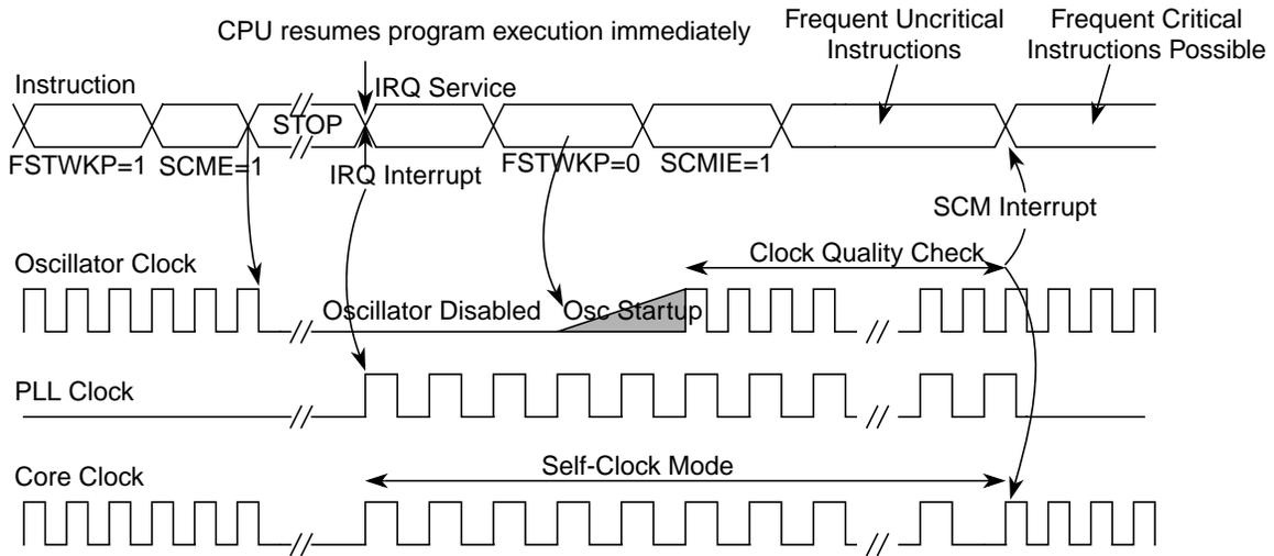
Figure 7-20. Fast Wake-up from Full Stop Mode: Example 2
