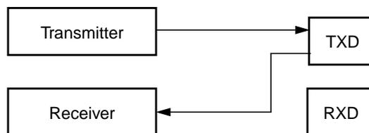
Figure 14-30. Single-Wire Operation (LOOPS = 1, RSRC = 1)
