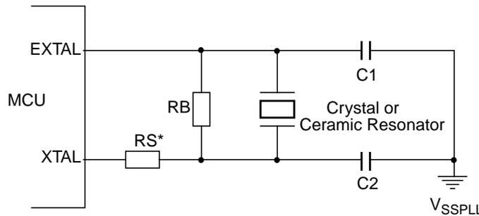
\*  $R_s$  can be zero (shorted) when use with higher frequency crystals. Refer to manufacturer's data.
