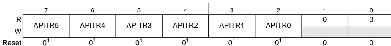
1. Reset value is either 0 or preset by factory. See Section 1 (Device Overview) for details.
