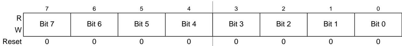
Figure 6-21. Debug Comparator Data Low Mask Register (DBGXDLM)
