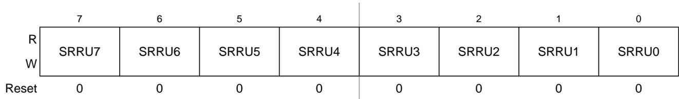
**Figure 2-84. Port U Polarity Select Register (SRRU)**
