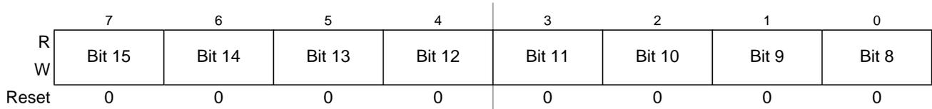
Figure 6-16. Debug Comparator Address Mid Register (DBGXAM)
