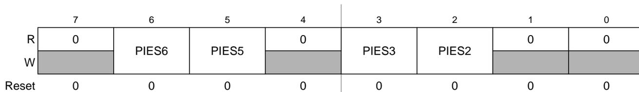
**Figure 2-72. Port S Interrupt Enable Register (PIES)**
