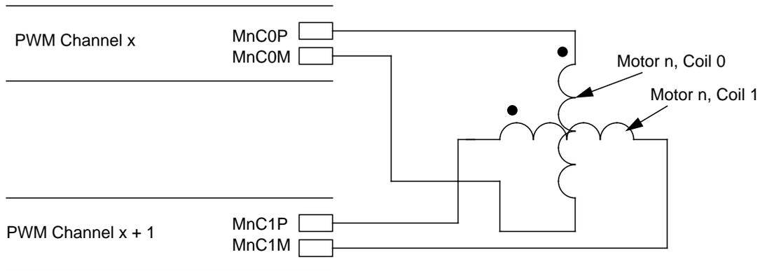
**Figure 20-10. Typical Dual Full H-Bridge Mode Configuration**
