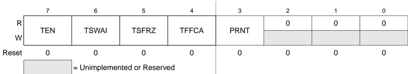
**Figure 16-12. Timer System Control Register 1 (TSCR1)**
