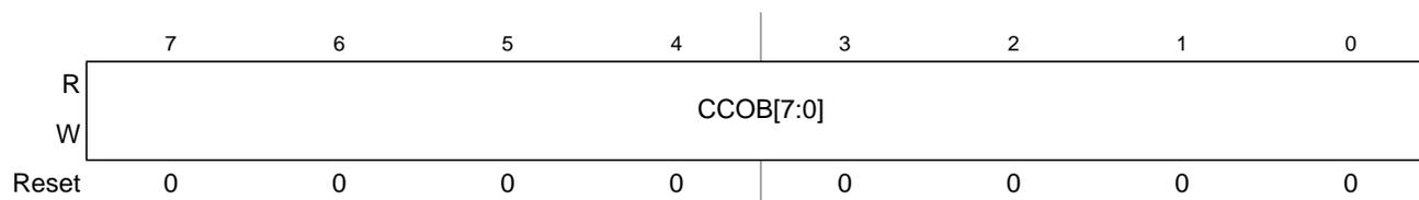
**Figure 19-17. Flash Common Command Object Low Register (FCCOBLO)**
