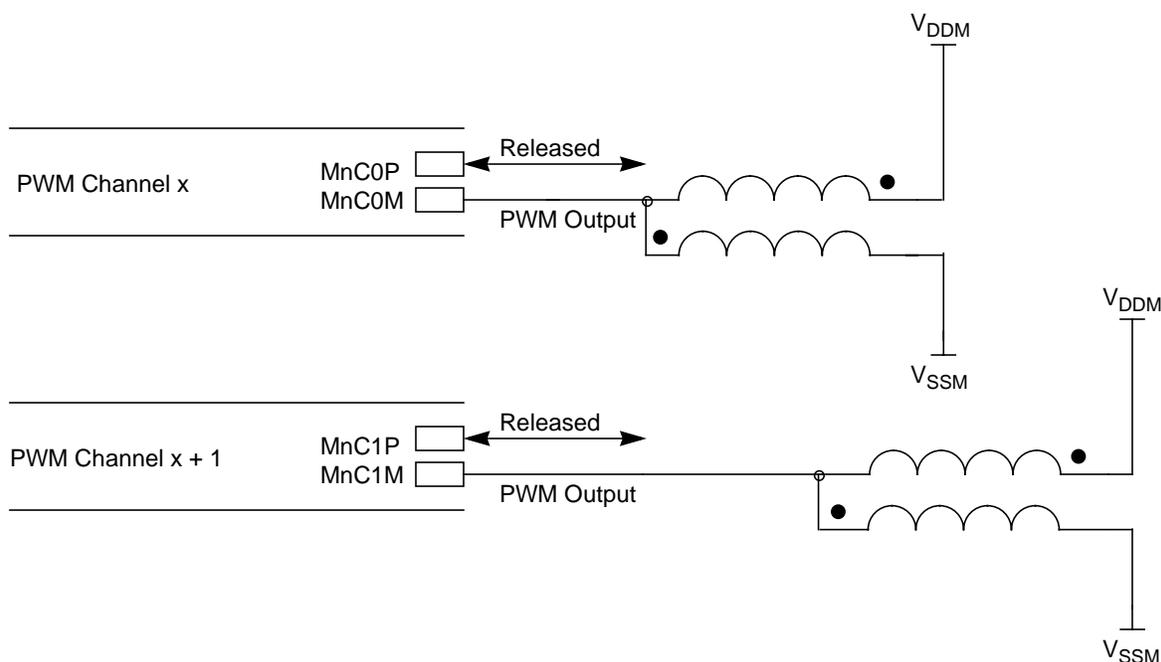
Figure 20-11. Typical Quad Half H-Bridge Mode Configuration
