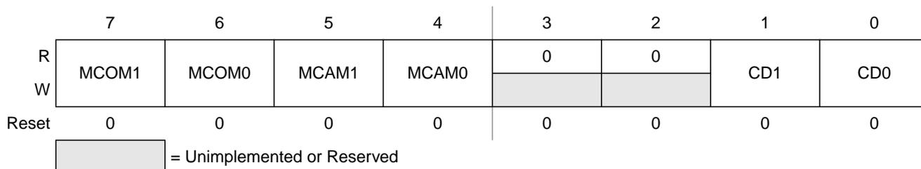
**Figure 20-7. Motor Controller Control Register Channel 0–7 (MCCC0–MCCC7)**
