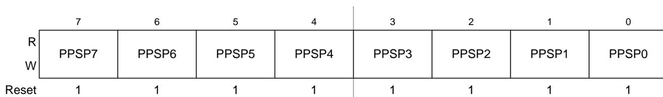
**Figure 2-41. Port P Polarity Select Register (PPSP)**
