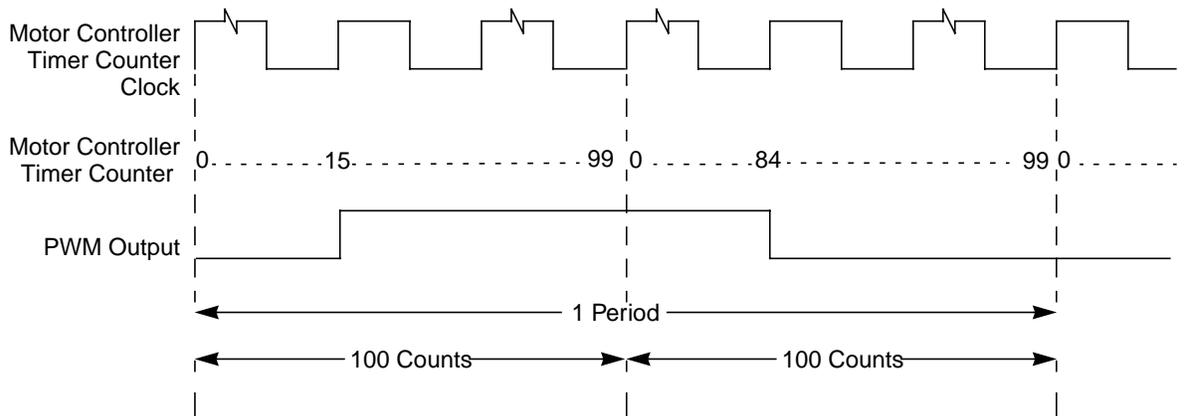
**Figure 20-21. PWM Output: DITH = 1, MCAM[1:0] = 11, MCDC = 31, MCPER = 200, RECIRC = 0**
