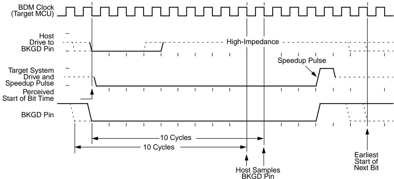
Figure 5-10. BDM Target-to-Host Serial Bit Timing (Logic 0)
