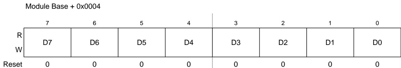
**Figure 12-8. IIC Bus Data I/O Register (IBDR)**
