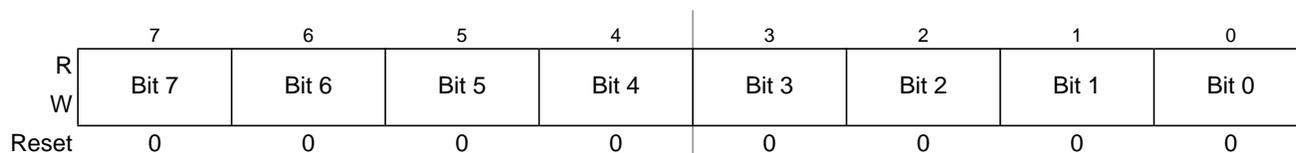
Figure 6-19. Debug Comparator Data Low Register (DBGXDL)
