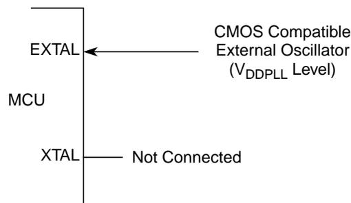
**Figure 8-4. External Clock Connections (FSP mode selected)**
