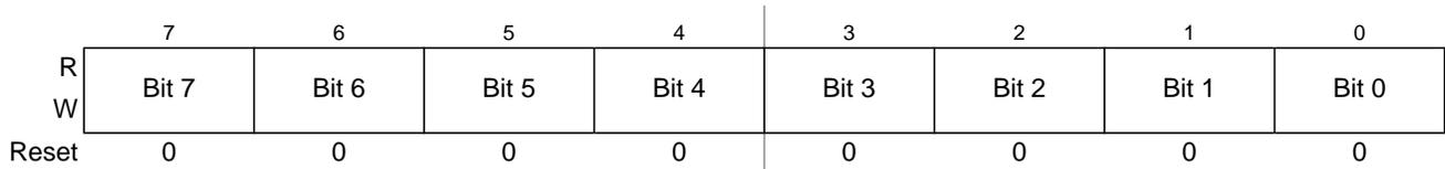
Figure 6-17. Debug Comparator Address Low Register (DBGXAL)
