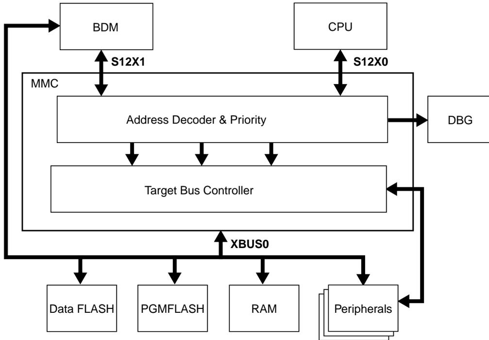
Figure 3-20. MMC Block Diagram
