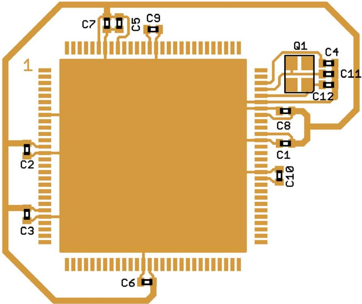
Figure C-1. 112-Pin LQFP Recommended PCB Layout (Loop Controlled Pierce Oscillator)
