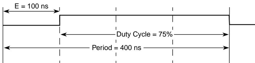
Figure 13-21. PWM Left Aligned Output Example Waveform
