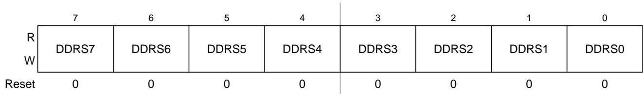
Figure 2-22. Port S Data Direction Register (DDRS)
