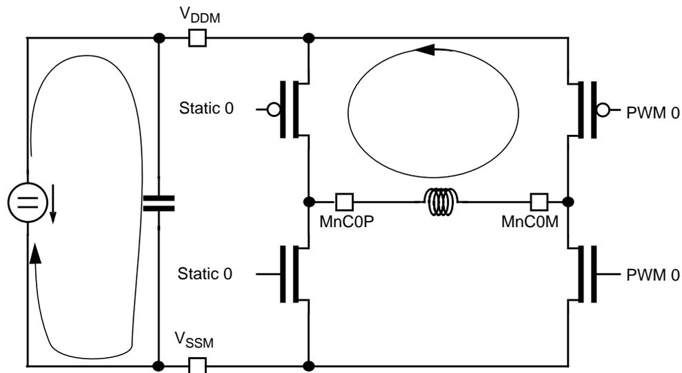
Figure 20-13. PWM Passive Phase, RECIRC = 0, S = 0
