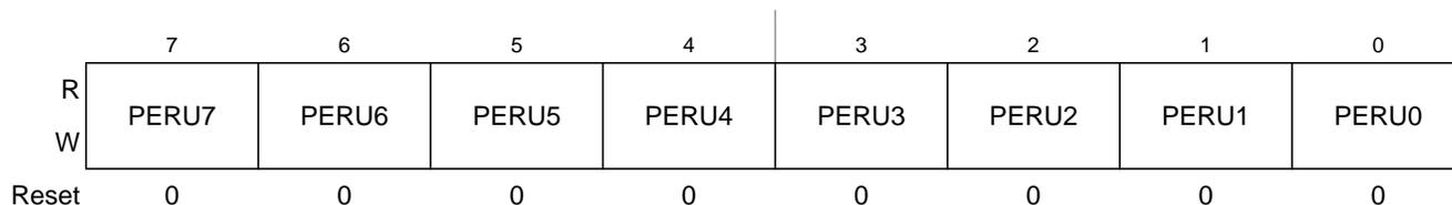
Figure 2-82. Port U Pull Device Enable Register (PERU)
