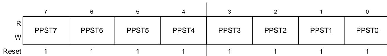
Figure 2-17. Port T Polarity Select Register (PPST)
