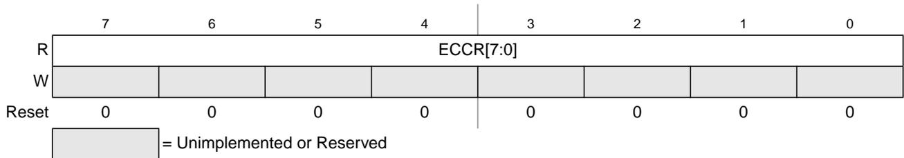
**Figure 18-21. Flash ECC Error Results Low Register (FECCRLO)**
