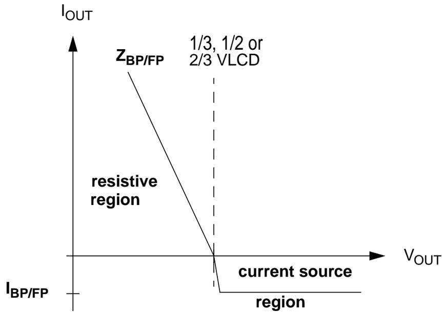
Figure A-8. buffer output characteristic
