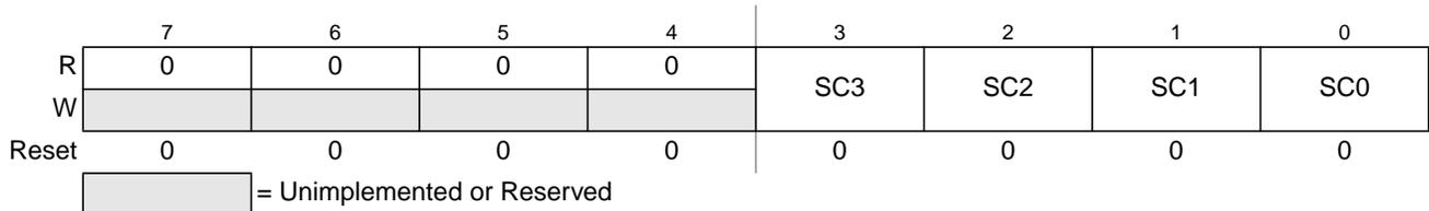
**Figure 6-10. Debug State Control Register 2 (DBGSCR2)**
