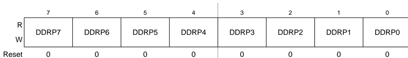
**Figure 2-38. Port P Data Direction Register (DDRP)**
