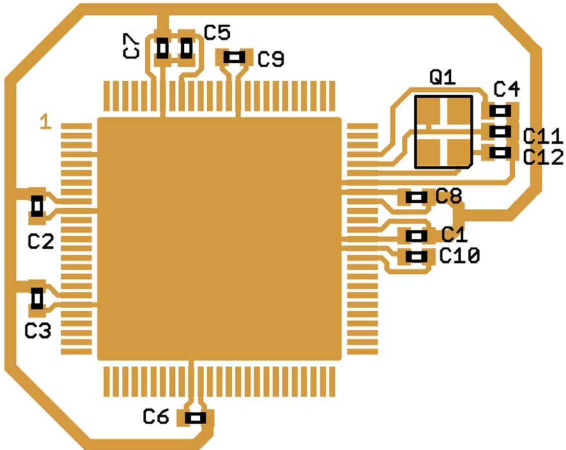
Figure C-2. 100-Pin QFP Recommended PCB Layout (Loop Controlled Pierce Oscillator)
