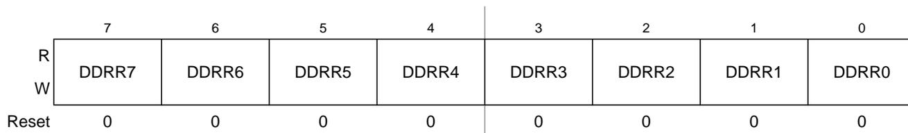
Figure 2-64. Port R Data Direction Register (DDRR)
