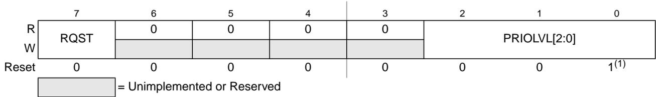
**Figure 4-10. Interrupt Request Configuration Data Register 4 (INT\_CFDATA4)**
