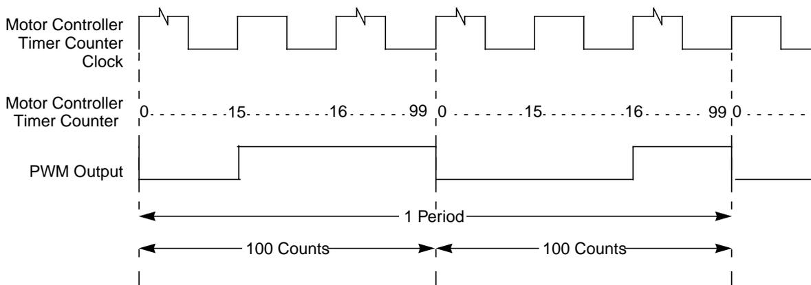
Figure 20-18. PWM Output: DITH = 1, MCAM[1:0] = 01, MCDC = 31, MCPER = 200, RECIRC = 0
