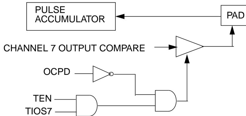
Figure 16-4. Channel 7 Output Compare/Pulse Accumulator Logic
