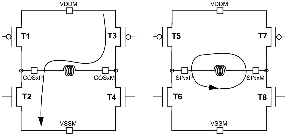
Figure 21-13. Current flow when STEP = 2, DCOIL = 1, ITG = 1
