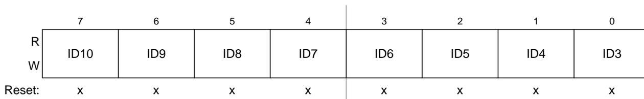
Figure 11-30. Identifier Register 0 — Standard Mapping
