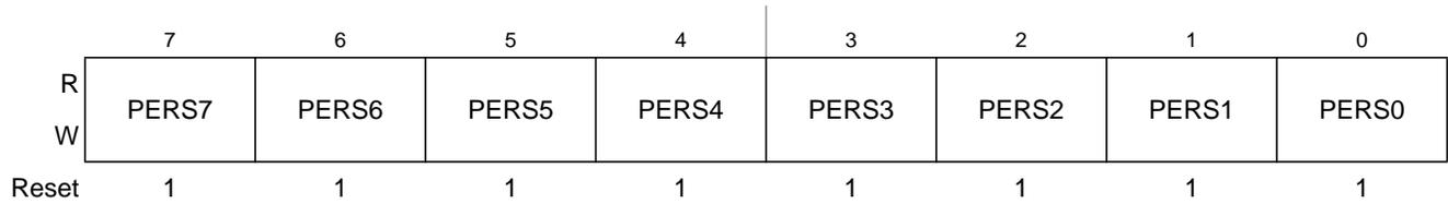
Figure 2-24. Port S Pull Device Enable Register (PERS)
