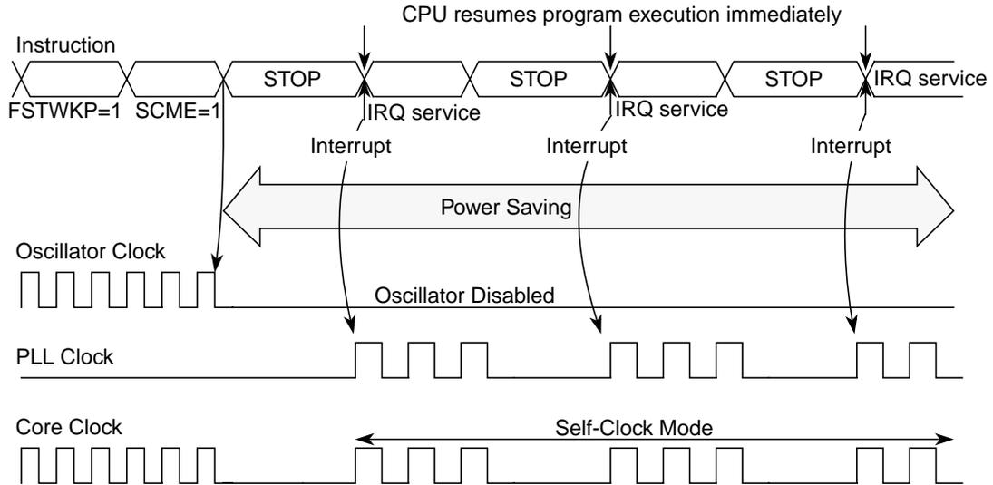
Figure 7-19. Fast Wake-up from Full Stop Mode: Example 1
