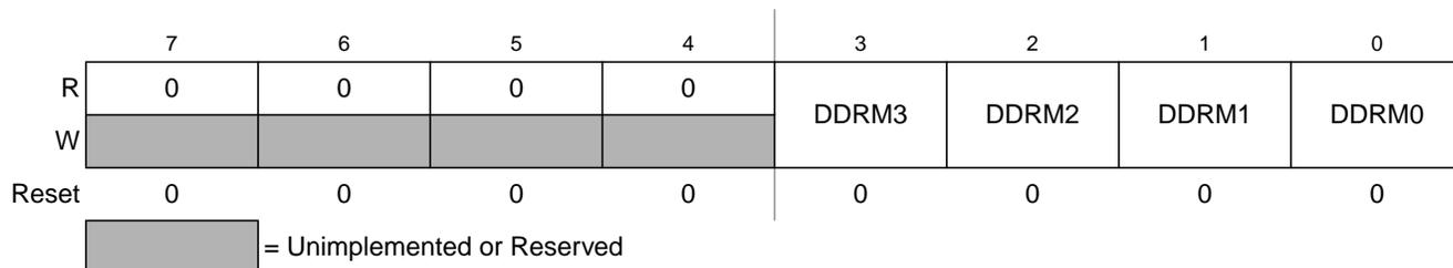
**Figure 2-30. Port M Data Direction Register (DDRM)**
