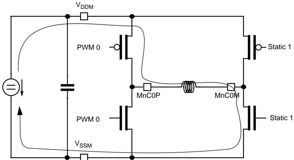
Figure 20-14. PWM Active Phase, RECIRC = 1, S = 0
