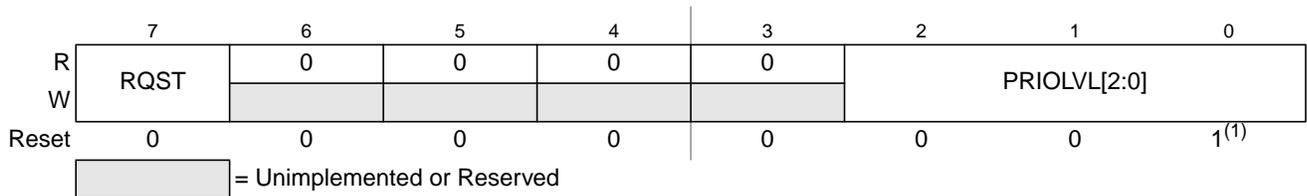
**Figure 4-12. Interrupt Request Configuration Data Register 6 (INT\_CFDATA6)**
