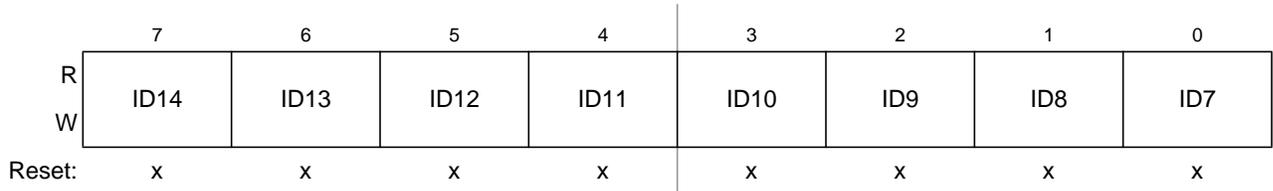
**Figure 11-28. Identifier Register 2 (IDR2) — Extended Identifier Mapping**
