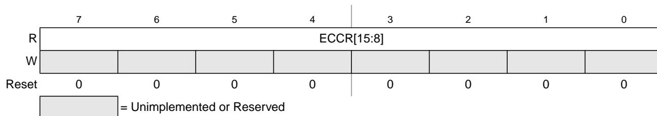
**Figure 19-20. Flash ECC Error Results High Register (FECCRHI)**
