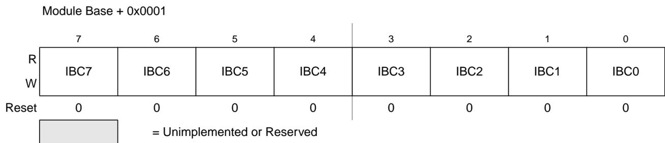
**Figure 12-4. IIC Bus Frequency Divider Register (IBFD)**
