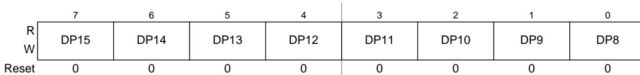
Figure 3-8. Direct Register (DIRECT)
