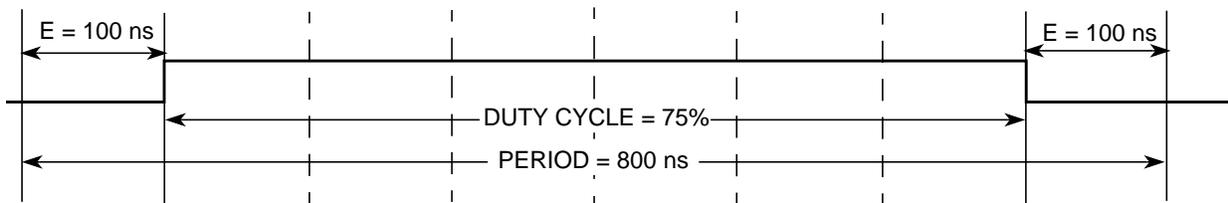
**Figure 13-23. PWM Center Aligned Output Example Waveform**
