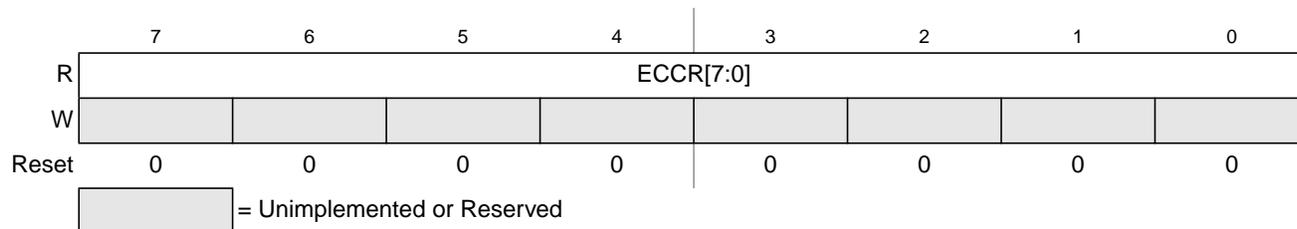
**Figure 19-21. Flash ECC Error Results Low Register (FECCRLO)**
