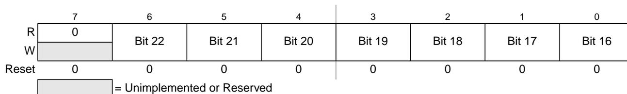
**Figure 6-15. Debug Comparator Address High Register (DBGXAH)**
