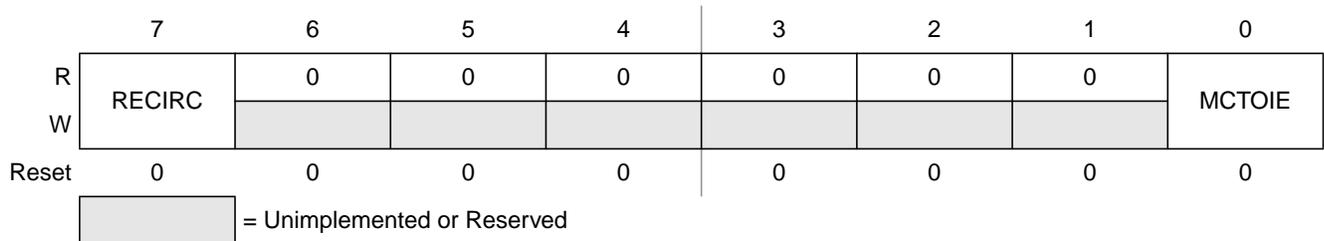
**Figure 20-4. Motor Controller Control Register 1 (MCCTL1)**
