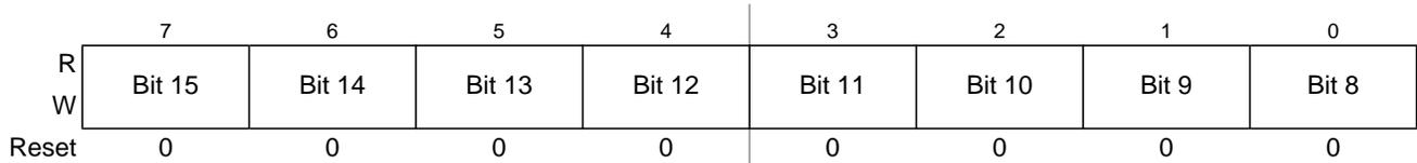
Figure 6-20. Debug Comparator Data High Mask Register (DBGXDHM)
