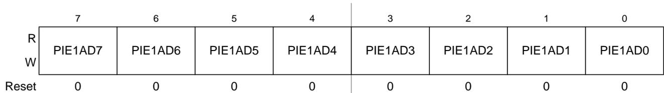
**Figure 2-74. Port AD Interrupt Enable Register (PIE1AD)**
