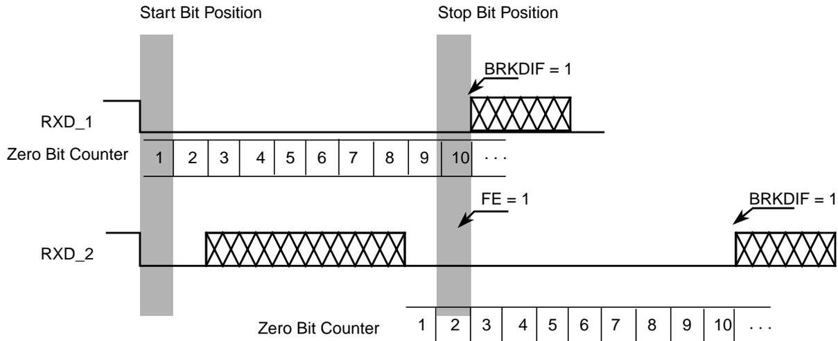
Figure 14-17. Break Detection if BRKDFE = 1 (M = 0)
