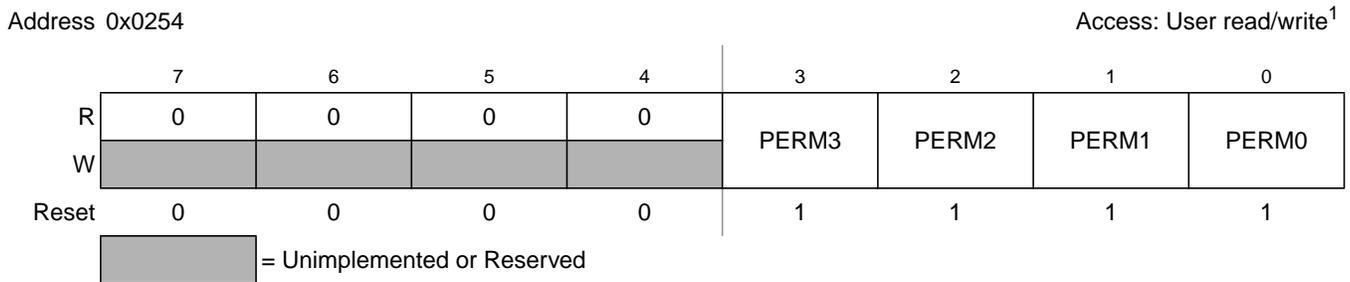
**Figure 2-32. Port M Pull Device Enable Register (PERM)**
