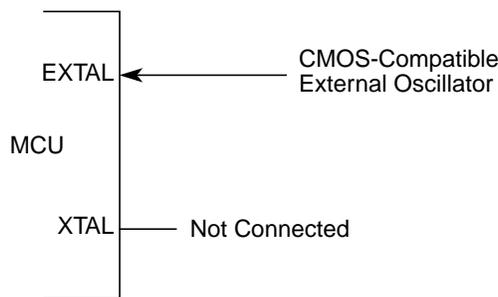
**Figure 1-8. External Clock Connections (XCLKS = 1)**
