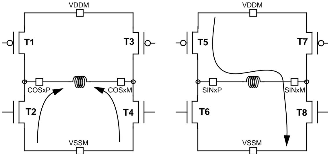
**Figure 21-12. Current Flow when STEP = 1, DCOIL = 1, ITG = 0, RCIR = 1**
