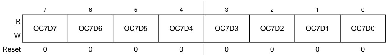
Figure 16-9. Output Compare 7 Data Register (OC7D)
