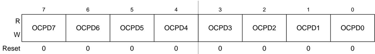
Figure 16-28. Ouput Compare Pin Disconnect Register (OCPD)
