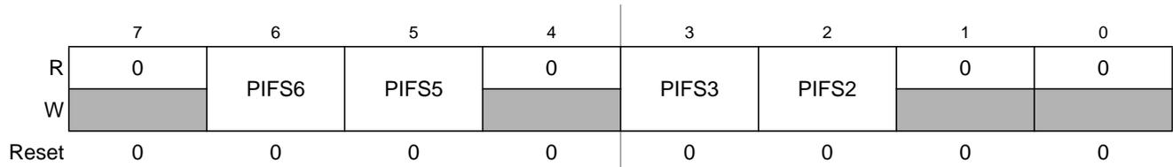
**Figure 2-73. Port S Interrupt Flag Register (PIFS)**
