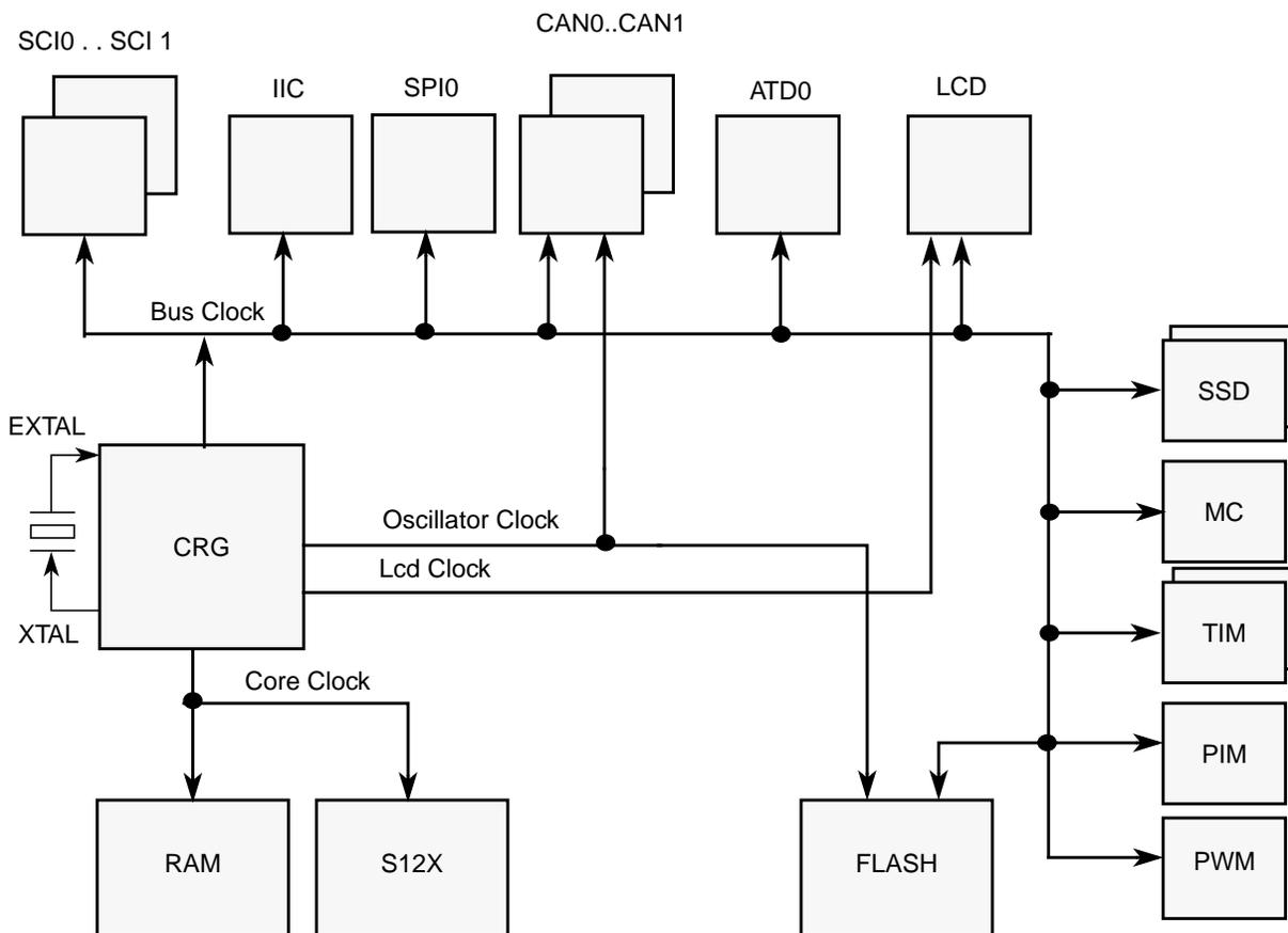
Figure 1-5. Clock Connections
