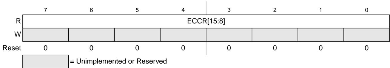
**Figure 18-20. Flash ECC Error Results High Register (FECCRHI)**
