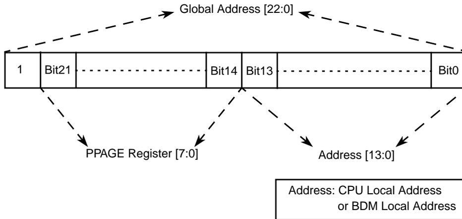
**Figure 3-12. PPAGE Address Mapping**
