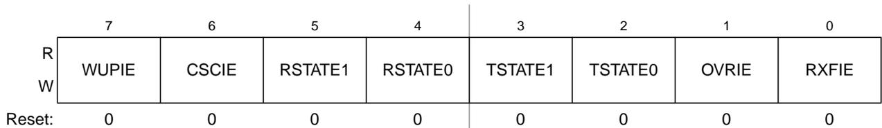
**Figure 11-9. MSCAN Receiver Interrupt Enable Register (CANRIER)**
