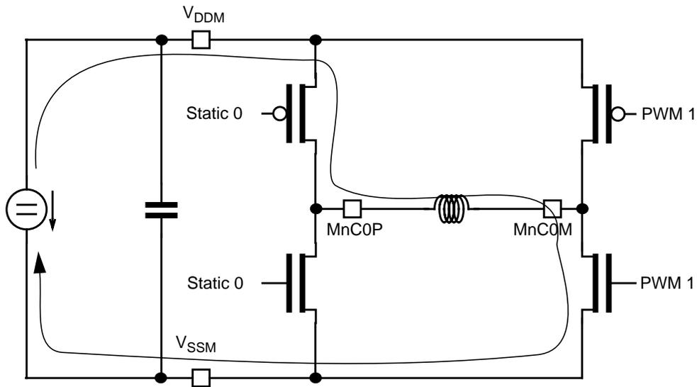
Figure 20-12. PWM Active Phase, RECIRC = 0, S = 0
