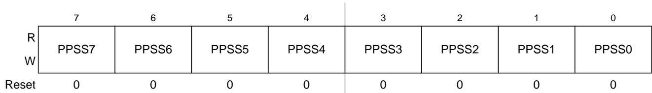
Figure 2-25. Port S Polarity Select Register (PPSS)
