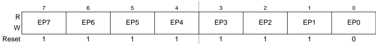
Figure 3-15. Data FLASH Page Index Register (EPAGE)
