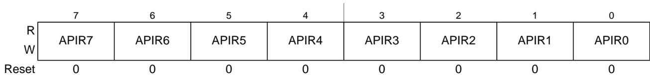
**Figure 9-6. Autonomous Periodical Interrupt Rate Low Register (VREGAPIRL)**
