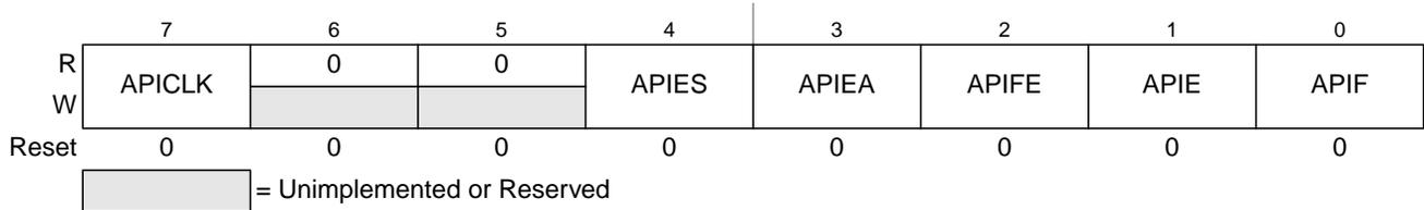
**Figure 9-3. Autonomous Periodical Interrupt Control Register (VREGAPICL)**
