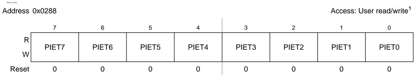
**Figure 2-70. Port T Interrupt Enable Register (PIET)**
