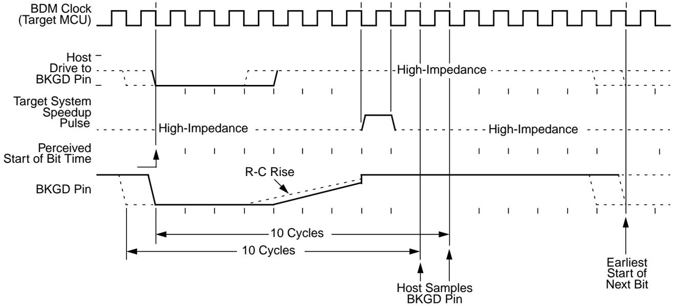
Figure 5-9. BDM Target-to-Host Serial Bit Timing (Logic 1)
