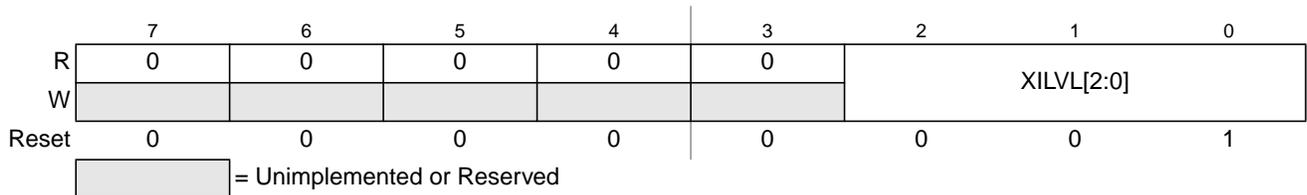
Figure 4-4. XGATE Interrupt Priority Configuration Register (INT\_XGPRIO)
