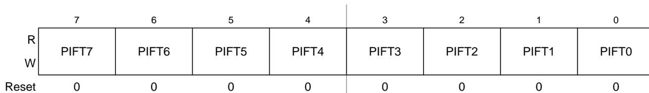
**Figure 2-71. Port T Interrupt Flag Register (PIFT)**
