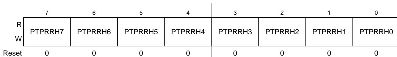
**Figure 2-42. Port P Routing Register High (PTPRRH)**
