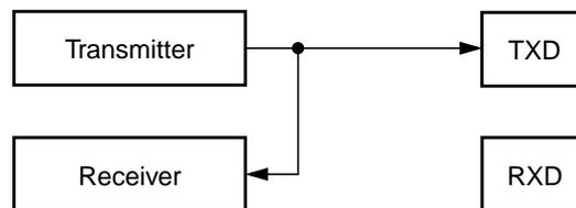
Figure 14-31. Loop Operation (LOOPS = 1, RSRC = 0)
