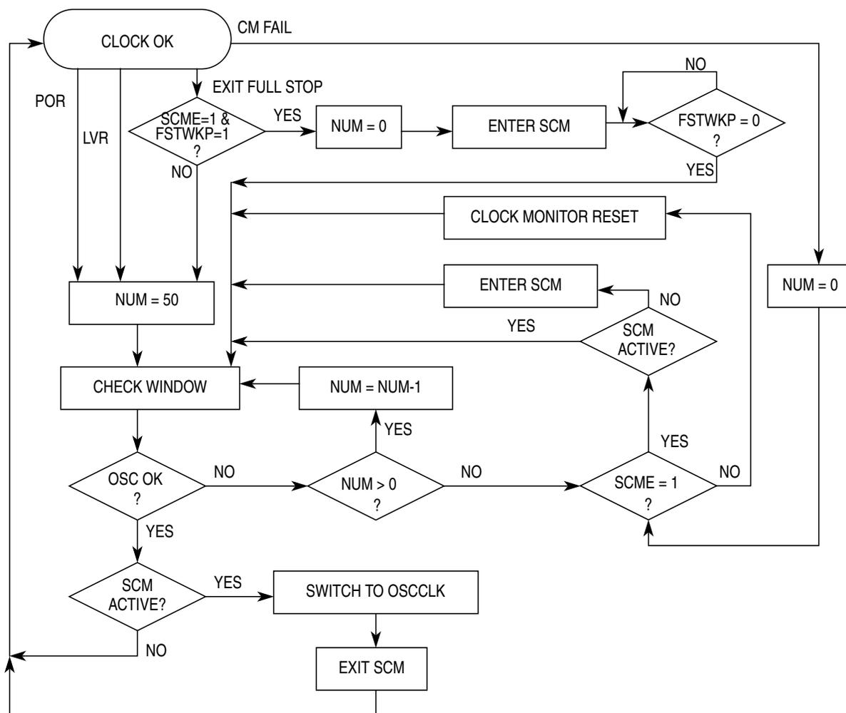
**Figure 7-18. Sequence for Clock Quality Check**
