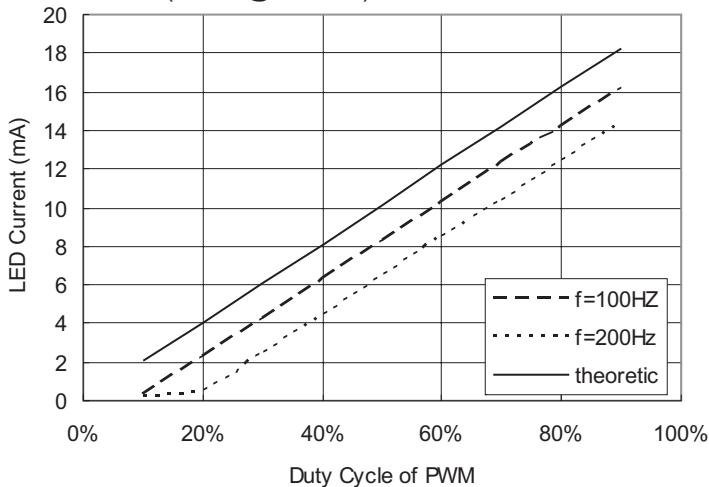
12. LED Current VS Duty Cycle of PWM
