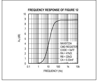
Figure 13. Increasing the Maximum Gain Using BassMax
