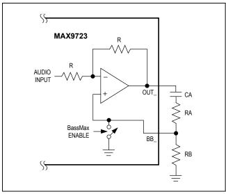
Figure 12. Using BassMax to Increase MAX9723's Maximum Gain
