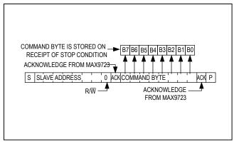
Figure 6. Write Data Format Example
