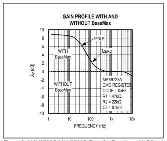
Figure 9. MAX9723C/MAX9723D Transfer Function with B5 = 1
