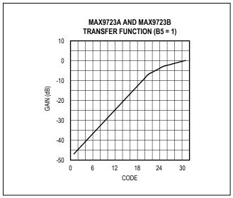
Figure 7. MAX9723A/MAX9723B Transfer Function with B5 = 1
