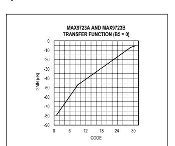
Figure 8. MAX9723A/MAX9723B Transfer Function with B5 = 0
