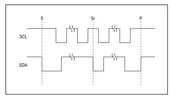
Figure 4. START, STOP, and REPEATED START Conditions
