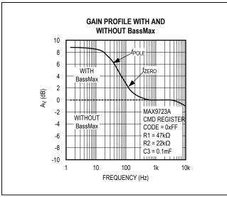
Figure 11. BassMax, Gain Profile Example
