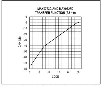
Figure 10. MAX9723C/MAX9723D Transfer Function with B5 = 0
