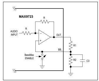
Figure 2. BassMax External Connections
