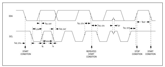
Figure 3. 2-Wire Serial-Interface Timing Diagram
