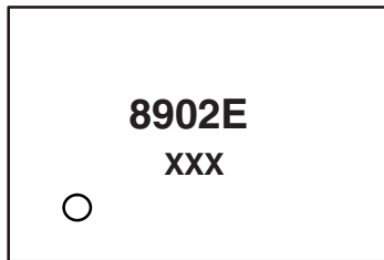
Mark on Backside of Die
