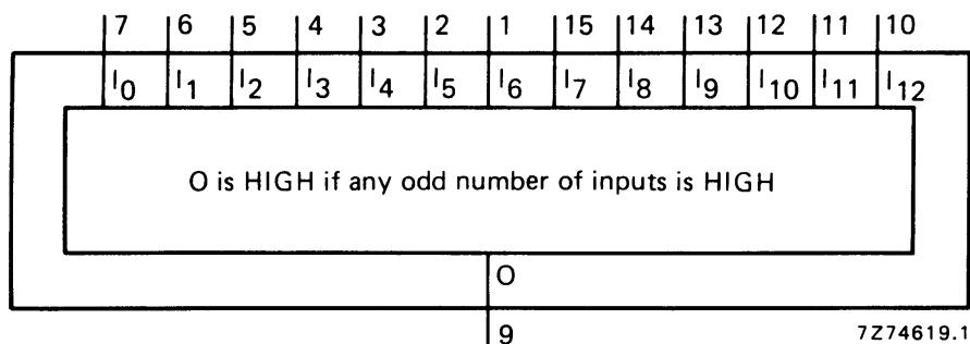
Fig.1 Functional diagram.
