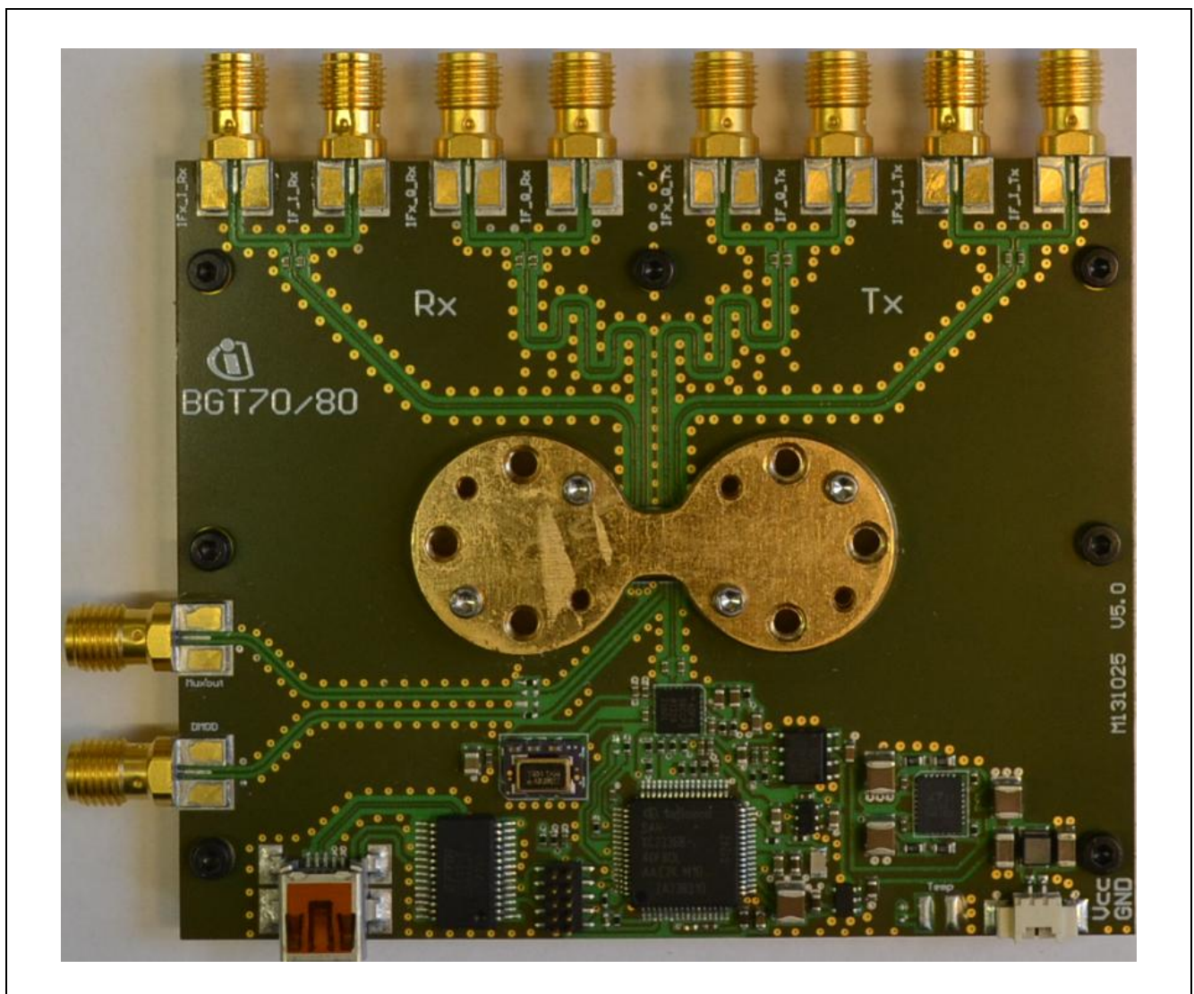
Figure 4 Evaluation Board for BGT80 – Top View
