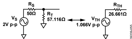
Figure 48. Thevenin Equivalent Circuit
