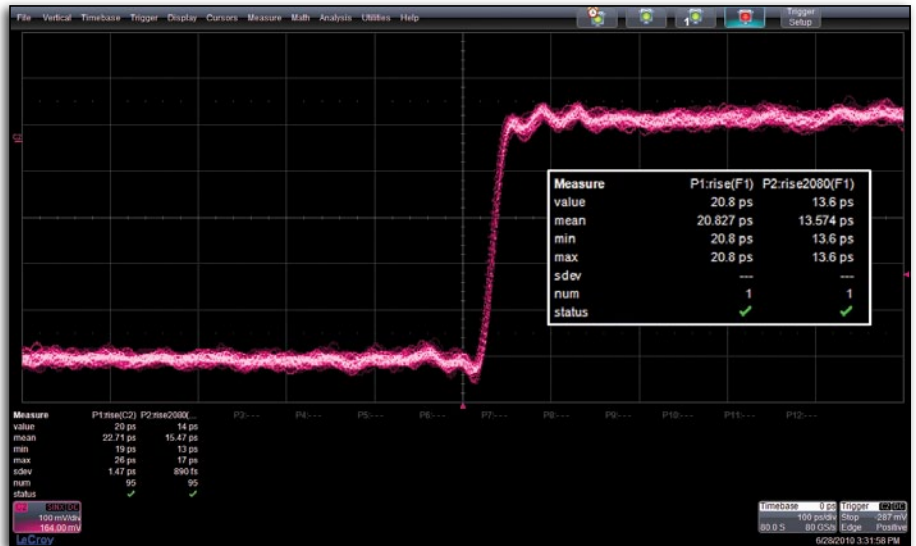
Teledyne LeCroy D2505-A probe with Dxx05-PT positioner (browser) tip showing rise time response with 20 ps differential input source.
