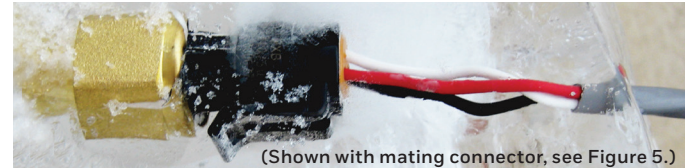
Figure 2. PX3 Series External Freeze/Thaw Resistance
