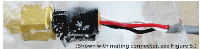
Figure 2. PX3 Series External Freeze/Thaw Resistance
