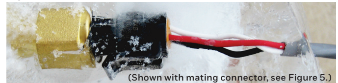
Figure 2. PX3 Series External Freeze/Thaw Resistance
