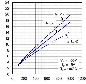
RATE OF CHANGE OF CURRENT :  $-di/dt(A/\mu s)$   $di/dt-I_{Rp}$  CHARACTERISTICS
