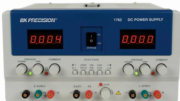
The 1760A series triple output DC power supplies offer three independent outputs with coarse and fine adjustment knobs for volts. The 4-digit LED display offers 10 mV and 1 mA resolution, providing the capability to set voltage and current values more accurately than 3-digit displays found in most comparable power supplies.
