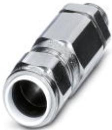
Cable gland, Cable gland material: Stainless steel 1.4404, Application: Ex, External cable diameter 40.4 mm ... 53.1 mm, Shielding: Yes, Connecting thread: M50, Color: silver
