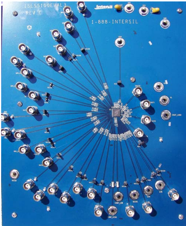
FIGURE 4. ISL55100A/BEVAL3/3Z EVALUATION BOARD
