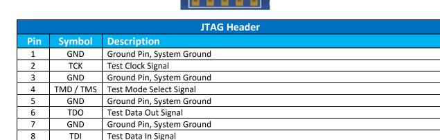
The JTAG header is used in the factory to program the bootloader into the BCM2835 SoC. It can also be used to connect to a compatible JTAG debugger, however should only be utilised by Advanced users who know what they are doing. This header makes for good mechanical support when adding a Daughter Board onto the Armadillo-70T, if nothing else.
