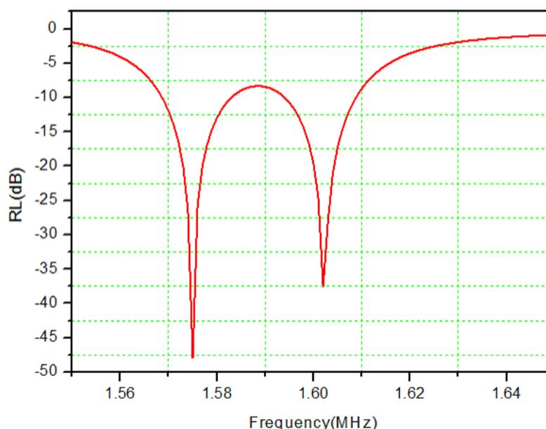
Return Loss characteristic shows a dual band response for GPS/Galileo & GLONASS
