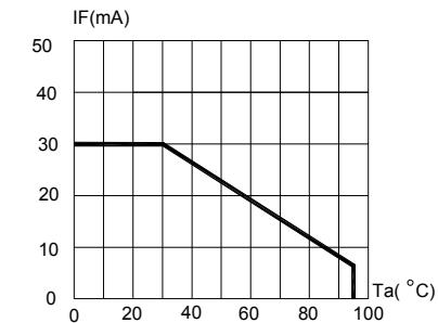
FIG.5 MAXIMUM FORWARD DC CURRENT
