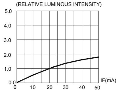
FIG.2 RELATIVE LUMINOUS INTENSITY VS.
