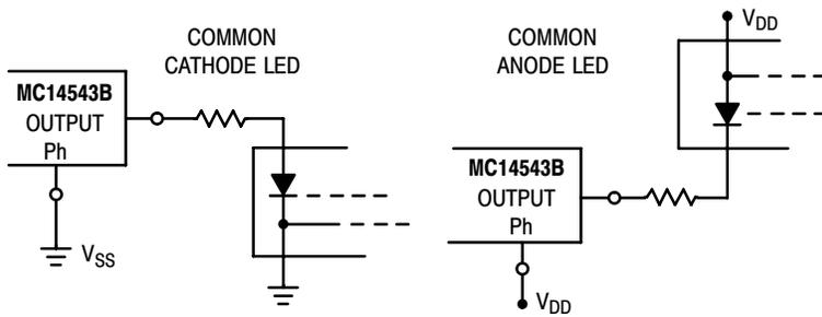
NOTE: Bipolar transistors may be added for gain (for  $V_{DD} \leq 10$  V or  $I_{out} \geq 10$  mA).
