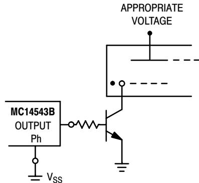
NOTE: Bipolar transistors may be added for gain (for  $V_{DD} \leq 10$  V or  $I_{out} \geq 10$  mA).
