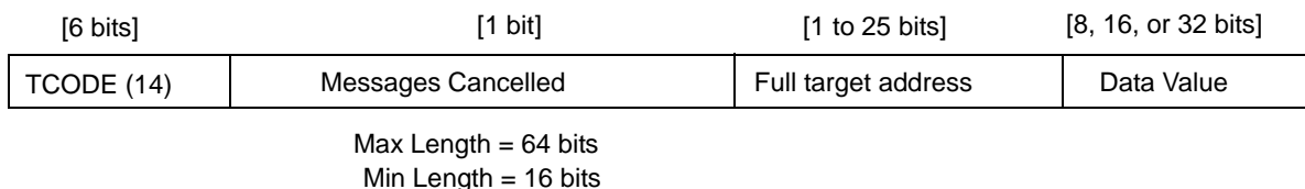
Figure 23-46. Data Read Synchronization Message Format
