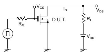
Fig.15 Switching Time Test Circuit
