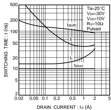
Fig.13 Switching characteristics
