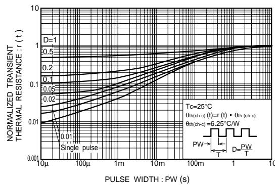
Fig.14 Normalized Transient Thermal Resistance vs . Pulse Width
