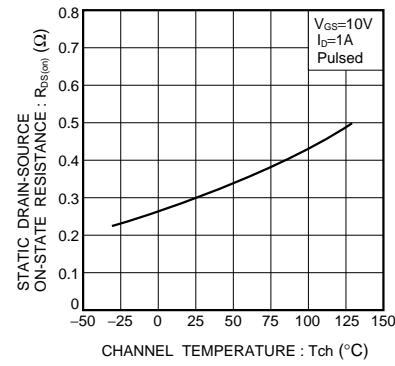
Fig.8 Static Drain-Source On-State Resistance vs. Channel Temperature
