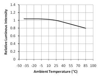
Figure 7. Relative luminous intensity versus ambient temperature.
