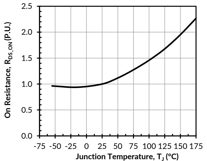
Figure 4. Normalized on-resistance vs. temperature at  $V_{GS} = 12V$  and  $I_D = 5A$
