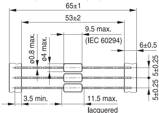
IND0429-B-E Minimum lead spacing 12.5 mm
