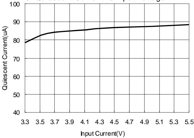
3. Quiescent Current vs Input Voltage
