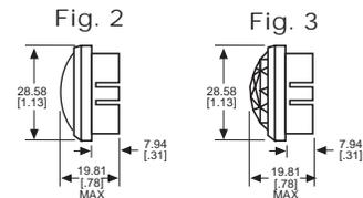
Material & Finish: Base - Nickel Plated Brass, Cap - Polycarbonate with Chrome Plated Brass Bezel
