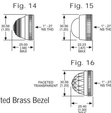
Material & Finish: Base - Nickel Plated Brass, Cap - Polycarbonate with Chrome Plated Brass Bezel
