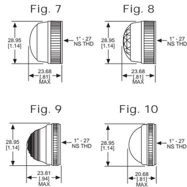
Material & Finish: Base - Chrome Plated Brass, Cap - Polycarbonate with Chrome Plated Brass Bezel
