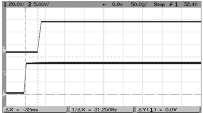
Startup Delay (Vin = 48V, Iout = 35A, Cout = 1000uF, Ta = +25°C) Ch1 = Vin, Ch2 = Vout
