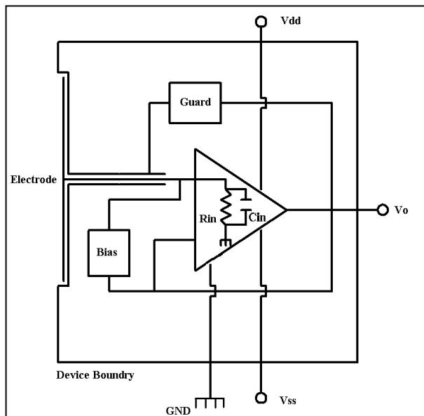
Fig. 2 Internal circuit of EPIC ECG Sensor
