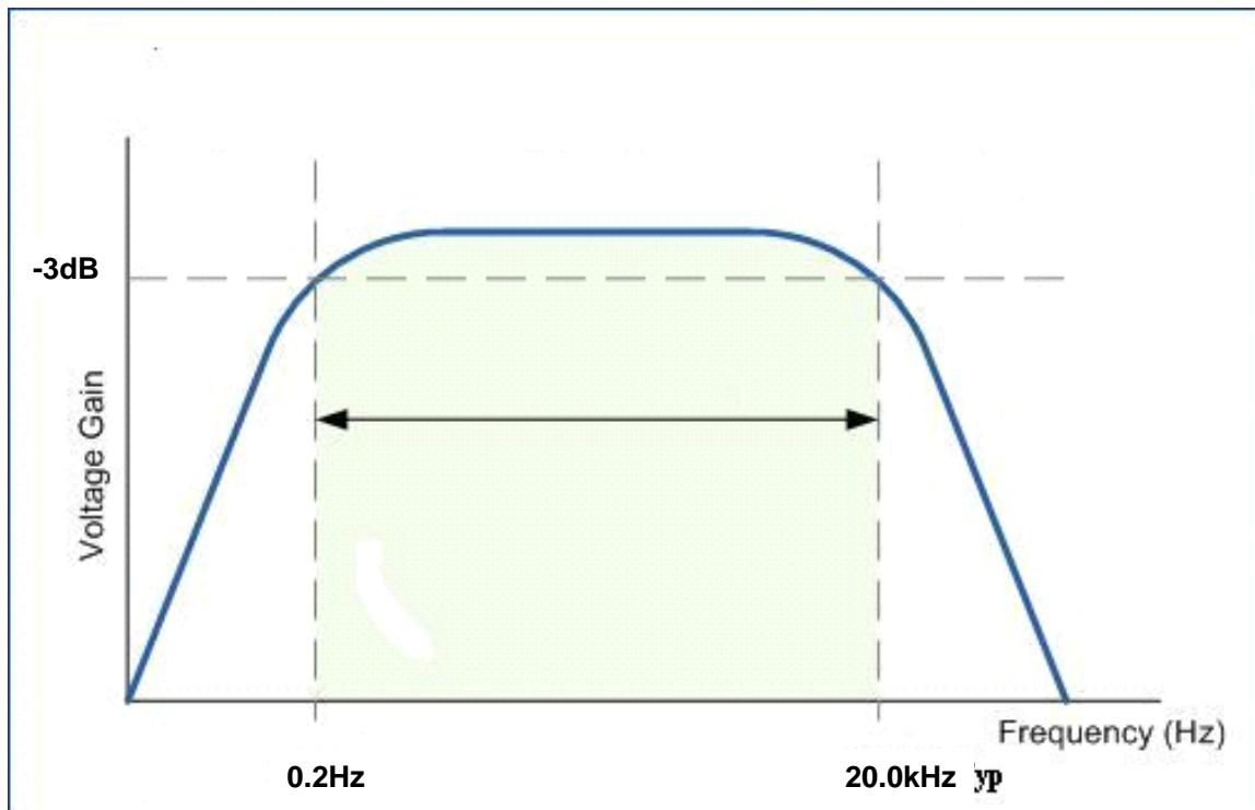
Fig. 3 Typical Bode Plot for EPIC ECG Sensor
