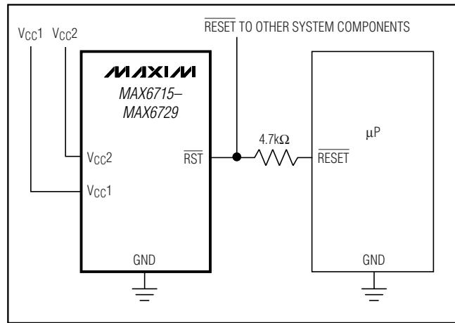
Figure 4. Interfacing to µPs with Bidirectional Reset I/O
