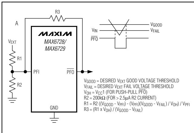
Figure 5. Adding Hysteresis to Power-Fail for Push-Pull PFO
