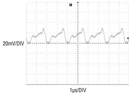
**Figure 3.** 3.3V Buck Output Ripple
