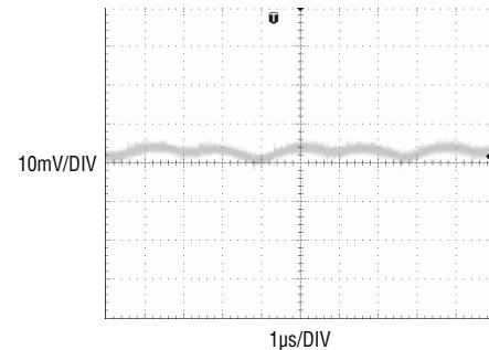
**Figure 4.** 2.5V LDO Output Ripple
