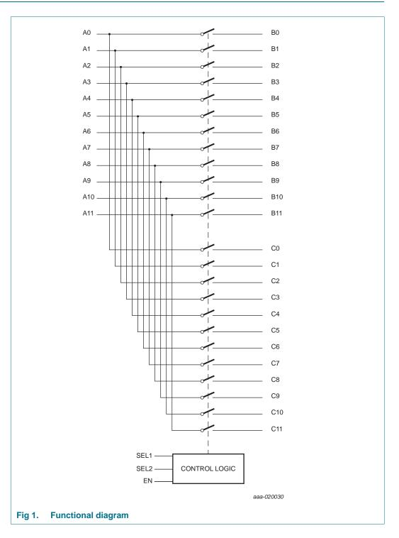
12-bit bus switch/multiplexer for DDR4-DDR3-DDR2 applications
