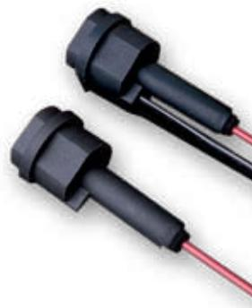
Fuse holders are rated up to 10 amperes at 300 volts and are equipped with 7" 18 AWG leads. Order part number LHR000 for two leads, and part number LHR001 for one lead; with the other terminal used for insertion of 18 AWG ballast lead.
