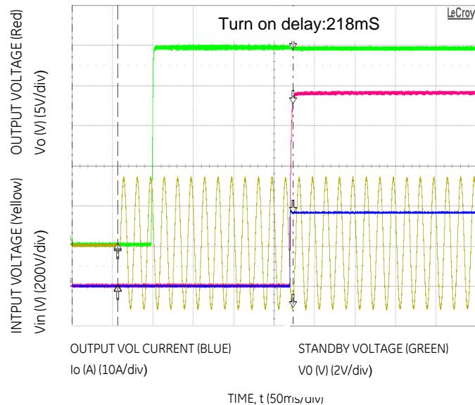
**Figure 5. Typical Start-up ( $V_{IN} = 230\text{Vac}$ , Full Load).**
