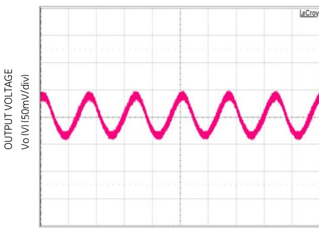
Figure 2. Typical output ripple and noise ( $V_{IN} = 230\text{Vac}$  100% load).
