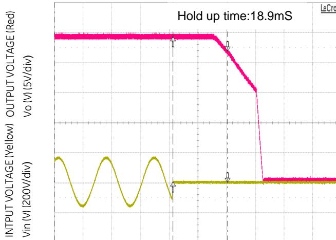
**Figure 6. Typical Hold-up waveforms ( $V_{IN} = 115\text{V}$ , 100% Load)**
