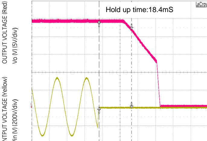
**Figure 7. Typical Hold-up waveforms ( $V_{IN} = 230\text{V}$ , 100% load)**
