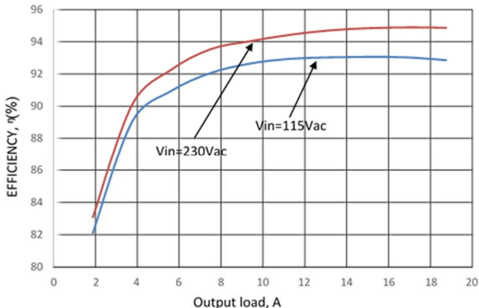
Figure 1. Power Supply Efficiency versus Output Current
