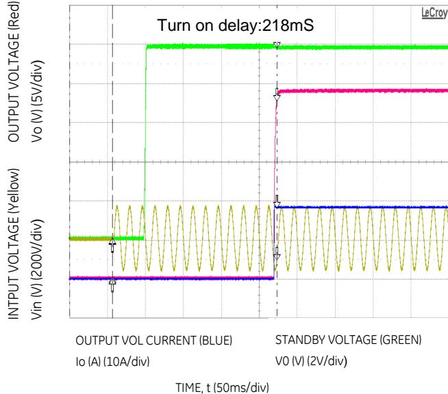
**Figure 4. Typical Start-up ( $V_{IN} = 115\text{Vac}$ , Full Load).**
