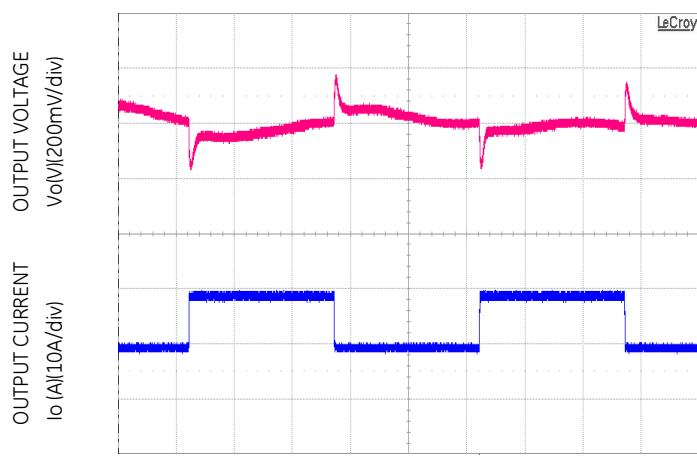
Figure 3. Transient Response to Dynamic Load change from 50% to 100% at  $V_{IN} = 230\text{Vac}$ .
