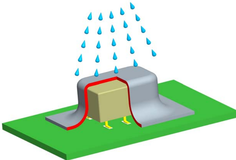
Fig. 4: Coating of relays on PCB's
