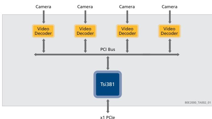
Figure 2 PC Digital Video Recorder Card Application
