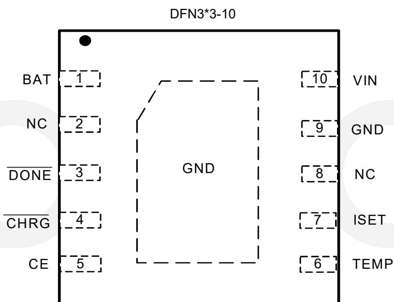
Figure 2 Pin Assignment
