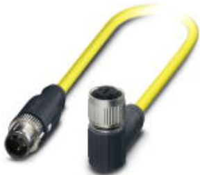
Sensor/Actuator cable, 3-position, PVC, Yellow RAL 1021, shielded, Plug straight M12-SPEEDCON, A-coded, on Socket angled M12-SPEEDCON, A-coded, Cable length: 0.5 m
