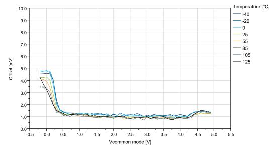
Figure 38-54. Offset vs.  $V_{CM}$  - 10 mV to 50 mV ( $V_{DD}$ =5V, T=25°C)
