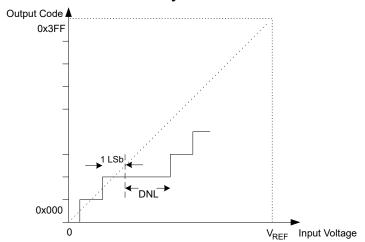
Quantization Error Due to the quantization of the input voltage into a finite number of codes, a range of input voltages (1 LSb wide) will code to the same value. Always ±0.5 LSb.
