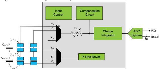
Figure 32-2. PTC Block Diagram Self Capacitance
