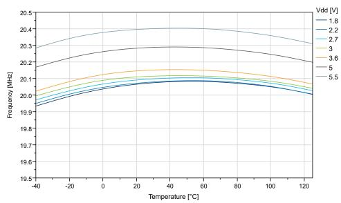
Figure 38-61. OSC20M Internal Oscillator: Frequency vs. Temperature
