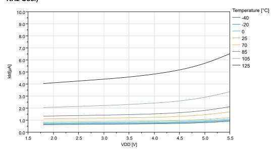
Figure 38-13. ATtiny1614 Standby Mode Supply Current vs.  $V_{DD}$  (RTC Running with Internal OSCULP32K)
