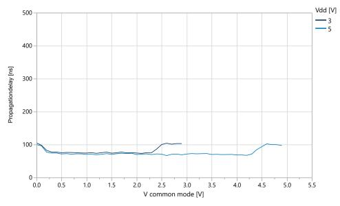
Figure 38-56. Propagation Delay vs.  $V_{CM}$  LPMODE Enabled, Rising Positive Input,  $V_{OD}$  = 30 mV (T=25°C)
