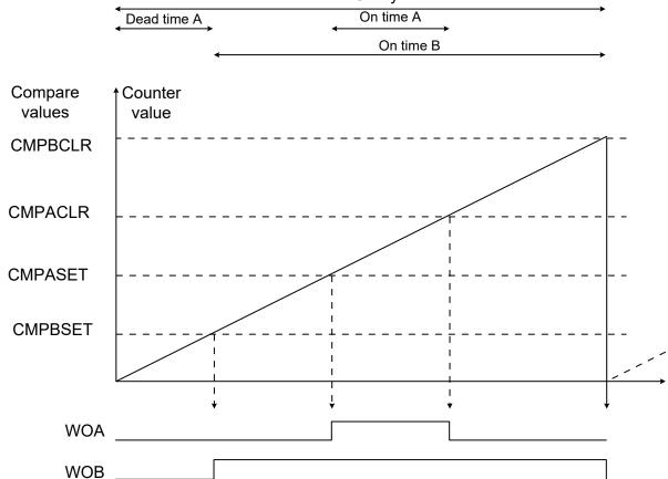
If any of the other compare values are bigger than CMPBCLR it will never be triggered when running in One Ramp mode, and if the CMPACLR is smaller than the CMPASET value, the clear value will not have any effect.
