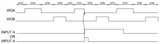
If Input mode 8 is used on input B and a positive input event occurs while in On-time B, the TCD counter jumps to Dead-time A.
