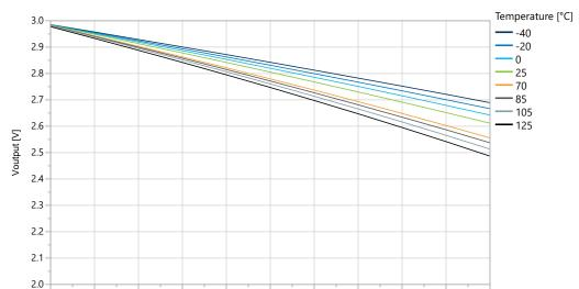
Figure 38-25. I/O Pin Output Voltage vs. Source Current (V<sub>DD</sub>=3.0V)
