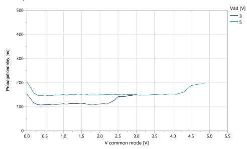
Figure 38-57. Propagation Delay vs.  $V_{CM}$  LPMODE Disabled, Falling Positive Input,  $V_{OD}$  = 30 mV (T=25°C)
