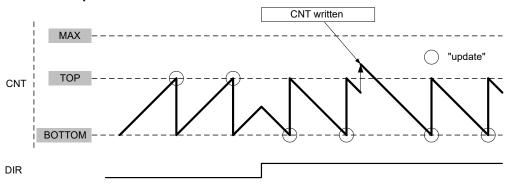
It is possible to change the counter value in the Counter register (TCAn.CNT) when the counter is running. The write access to TCAn.CNT has higher priority than count, clear, or reload, and will be immediate. The direction of the counter can also be changed during normal operation by writing to DIR in TCAn.CTRLE.
