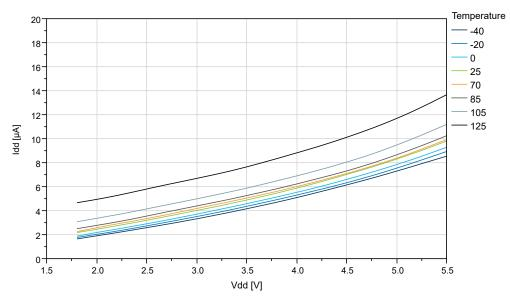
Figure 38-9. ATtiny1614 Idle Supply Current vs. V<sub>DD</sub> (f=32 KHz OSCULP32K)
