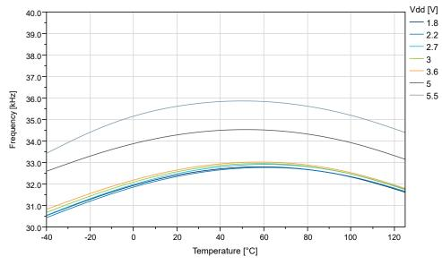
Figure 38-64. OSCULP32K Internal Oscillator Frequency vs. V<sub>DD</sub>
