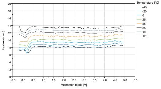
Figure 38-52. Hysteresis vs.  $V_{CM}$  - 10 mV to 50 mV ( $V_{DD}$ =5V, T=25°C)
