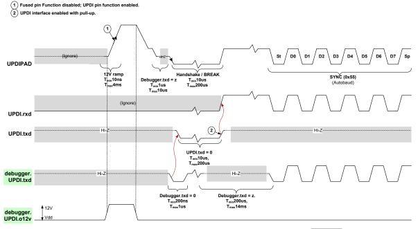
When enabled by 12V, only a POR will disable the UPDI configuration on the RESET pin, and restore the default setting. If issuing a UPDI Disable command through the UPDIDIS bit in UPDI.CTRLB, the UPDI will be reset and the clock request will be canceled, but the RESET pin will remain in UPDI configuration.
