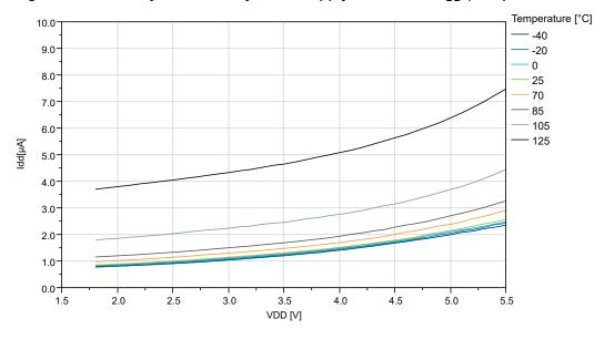
Figure 38-15. ATtiny1614 Standby Mode Supply Current vs. V<sub>DD</sub> (Sampled BOD Running at 1 kHz)
