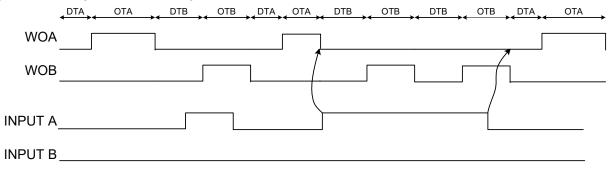
If Input mode 3 is used on input B, an event will only have an effect if the TCD is in Dead-time B or Ontime B.
