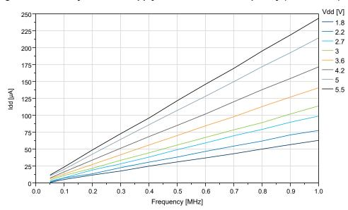
Figure 38-7. ATtiny1614 Idle Supply Current vs. Low Frequency (0.1-1.0 MHz) at T=25°C
