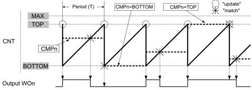
The TCAn.PER register defines the PWM resolution. The minimum resolution is 2 bits (TCA.PER=0x0003), and the maximum resolution is 16 bits (TCA.PER=MAX).
