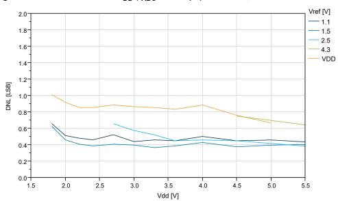
Figure 38-43. DNL Error vs.  $V_{DD}$  ( $f_{ADC}$ =115 ksps) at T=25°C, REFSEL = Internal Reference
