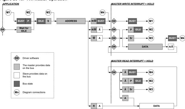
The number of interrupts generated is kept to a minimum by an automatic handling of most conditions.
