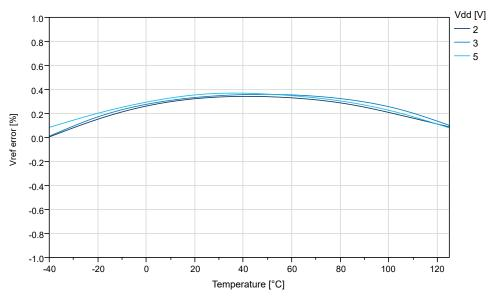
Figure 38-32. Internal 1.1V Reference vs. Temperature
