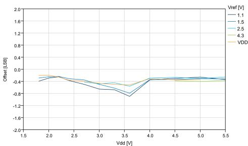
Figure 38-49. Offset Error vs.  $V_{DD}$  ( $f_{ADC}$ =115 ksps) at T=25°C, REFSEL = Internal Reference
