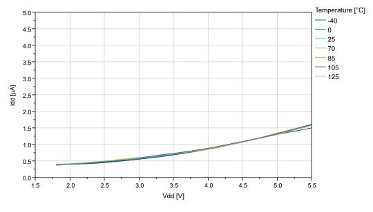
Figure 38-37. BOD Current vs. V<sub>DD</sub> (Sampled BOD at 1 kHz)
