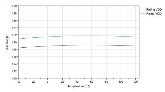
Figure 38-39. BOD Threshold vs. Temperature (Level 2.6V)
