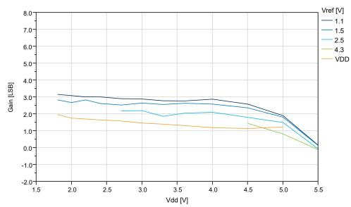
Figure 38-45. Gain Error vs.  $V_{DD}$  ( $f_{ADC}$ =115 ksps) at T=25°C, REFSEL = Internal Reference
