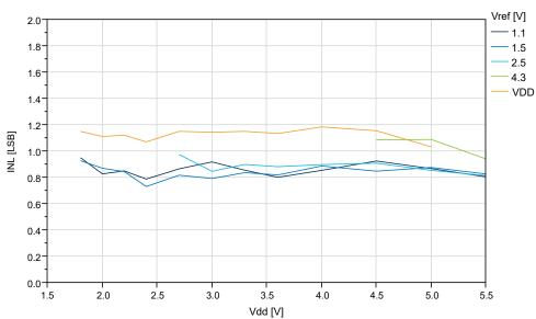
Figure 38-47. INL vs. V<sub>DD</sub> (f<sub>ADC</sub>=115 ksps) at T=25°C, REFSEL = Internal Reference
