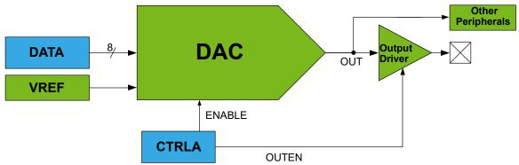
**Note:** Only DAC0 has an output driver for an external pin.
