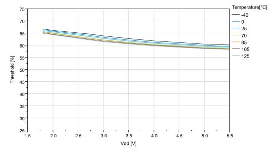
Figure 38-19. I/O Pin Input Threshold Voltage vs.  $V_{DD}$  ( $V_{IL}$ )
