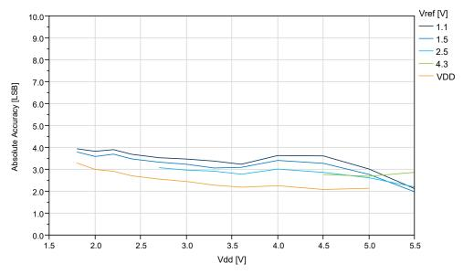
Figure 38-42. Absolute Accuracy vs.  $V_{ref}$  ( $V_{DD}$ =5.0V,  $f_{ADC}$ =115 ksps), REFSEL = Internal Reference
