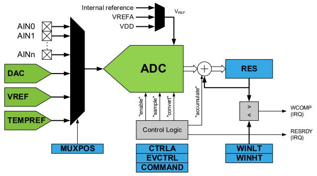
The analog input channel is selected by writing to the MUXPOS bits in the MUXPOS register (ADC.MUXPOS). Any of the ADC input pins, GND, or temperature sensor, can be selected as single-ended input to the ADC. The ADC is enabled by writing a '1' to the ADC ENABLE bit in the Control A register (ADC.CTRLA). Voltage reference and input channel selections will not go into effect before the ADC is enabled. The ADC does not consume power when the ENABLE bit in ADC.CTRLA is '0'.
