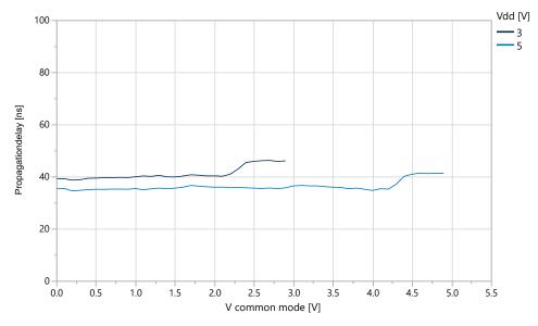
Figure 38-58. Propagation Delay vs.  $V_{CM}$  LPMODE Disabled, Rising Positive Input,  $V_{OD}$  = 30 mV (T=25°C)
