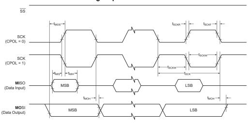
Table 37-17. USART in SPI Master Mode - Timing Characteristics
