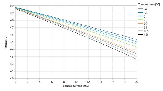
Figure 38-27. I/O Pin Output Voltage vs. Source Current (T=25°C)
