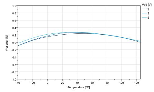
Figure 38-33. Internal 2.5V Reference vs. Temperature
