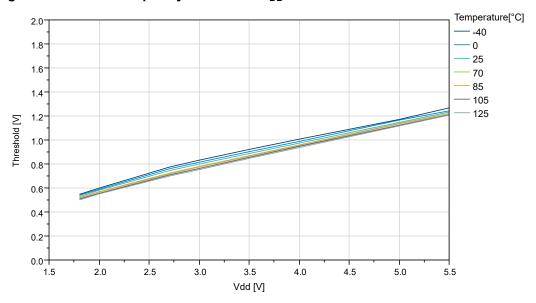
Figure 38-17. I/O Pin Input Threshold Voltage vs. V<sub>DD</sub> (T=25°C)
