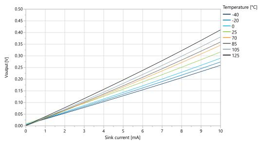
Figure 38-21. I/O Pin Output Voltage vs. Sink Current (V<sub>DD</sub>=3.0V)
