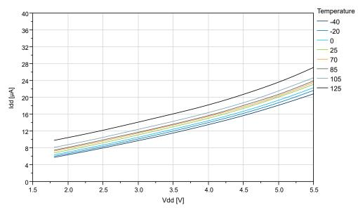
Figure 38-5. ATtiny1614 Active Supply Current vs. V<sub>DD</sub> (f=32 KHz OSCULP32K)
