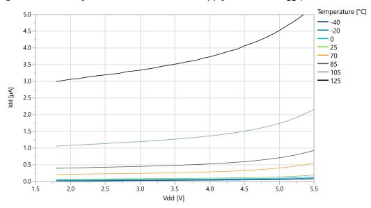
Figure 38-11. ATtiny1614 Power-Down Mode Supply Current vs. V<sub>DD</sub> (all functions disabled)
