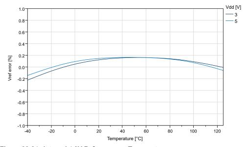
Figure 38-34. Internal 4.3V Reference vs. Temperature
