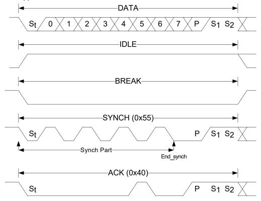
Data Frame Data frame consists of one Start bit (always low), eight data bits, one parity bit (even parity), and two Stop bits (always high). If the Start bit, parity bit, or Stop bits have an incorrect value, an error will be detected and signalized by the UPDI. The parity bit-check in the UPDI can be disabled by writing the PARD bit in UPDI.CTRLA, in which case the parity generation from the debugger can be ignored.
