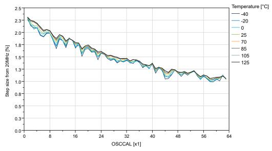
Figure 38-60. OSC20M Internal Oscillator: Frequency vs. Calibration Value (V<sub>DD</sub>=3V)
