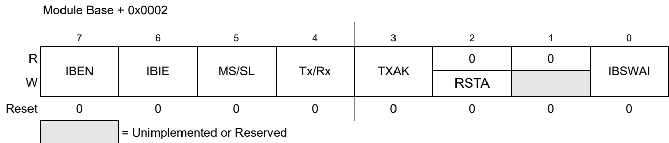
Figure 20-6. IIC Bus Control Register (IBCR)
