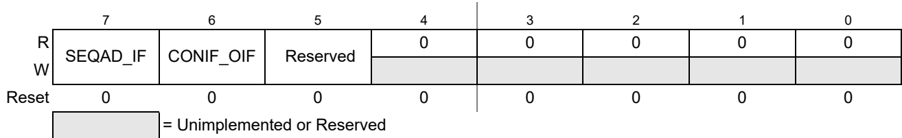
Figure 10-13. ADC Interrupt Flag Register (ADCIF)
