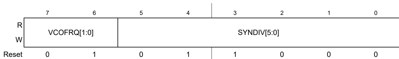
Figure 9-7. S12CPMU_UHV Synthesizer Register (CPMUSYNR)
