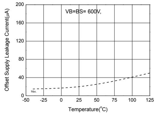
Figure 13a. Offset Supply Leakage Current vs Temperature
