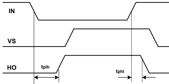
Figure 1. Input /output Timing Diagram
