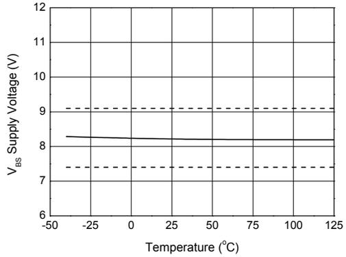
Figure 19b. VBS Under voltage Threshold(-) vs Temperature
