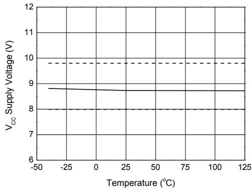
Figure 18a. VCC Under voltage Threshold(+) vs Temperature
