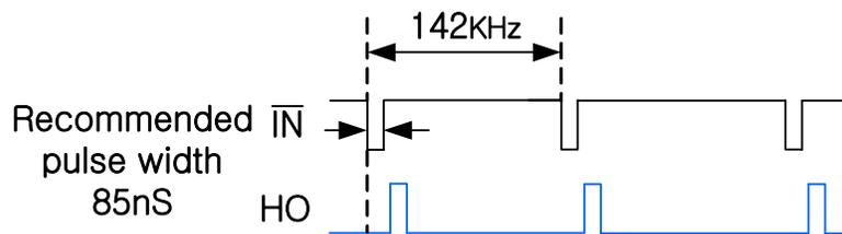
Figure 4c. Recommendation of pulse width Output Waveform
