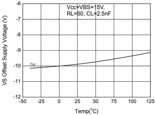
Figure 22a. Maximum VS Negative Voltage vs Temperature
