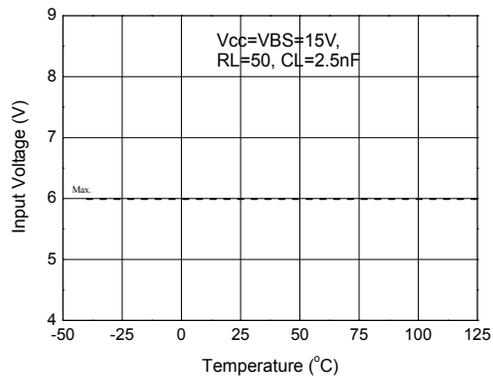
Figure 10a. Logic "0" IN Voltage vs Temperature
