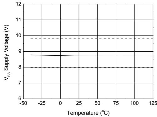
Figure 19a. VBS Under voltage Threshold(+) vs Temperature
