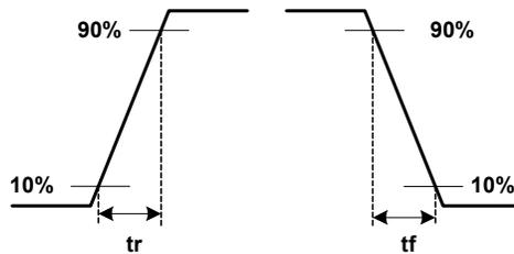
Figure 2. Switching Time Waveform Definitions
