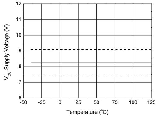
Figure 18b. VCC Under voltage Threshold(-) vs Temperature
