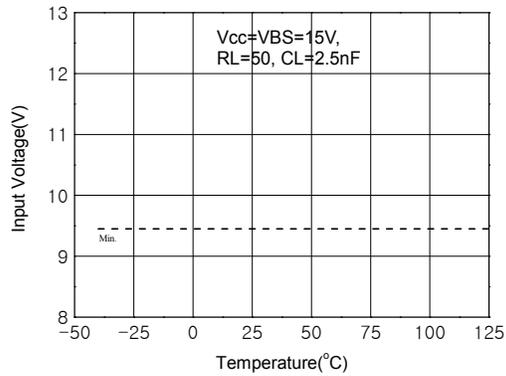
Figure 9a. Logic "1" IN Voltage vs Temperature
