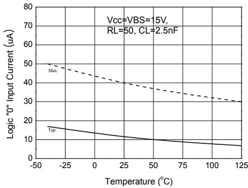
Figure 16a. Logic "0" IN Current vs Temperature
