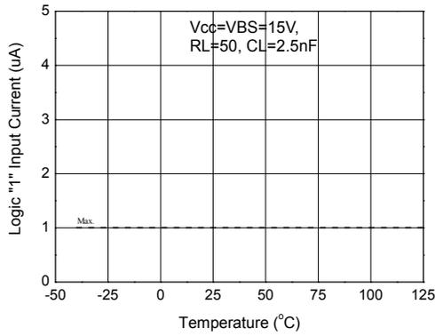
Figure 17a. Logic "1" IN Current vs Temperature
