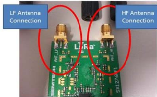
Figure 6: LF and HF Antenna Connection
