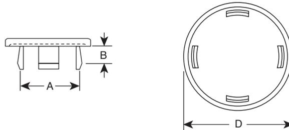
Economical snap-in Poly-Plugs will close unneeded chassis holes, wiring outlets, fill unused accessory openings, cover inspection and production access holes. They can be used as tube end caps and protective bumpers.
