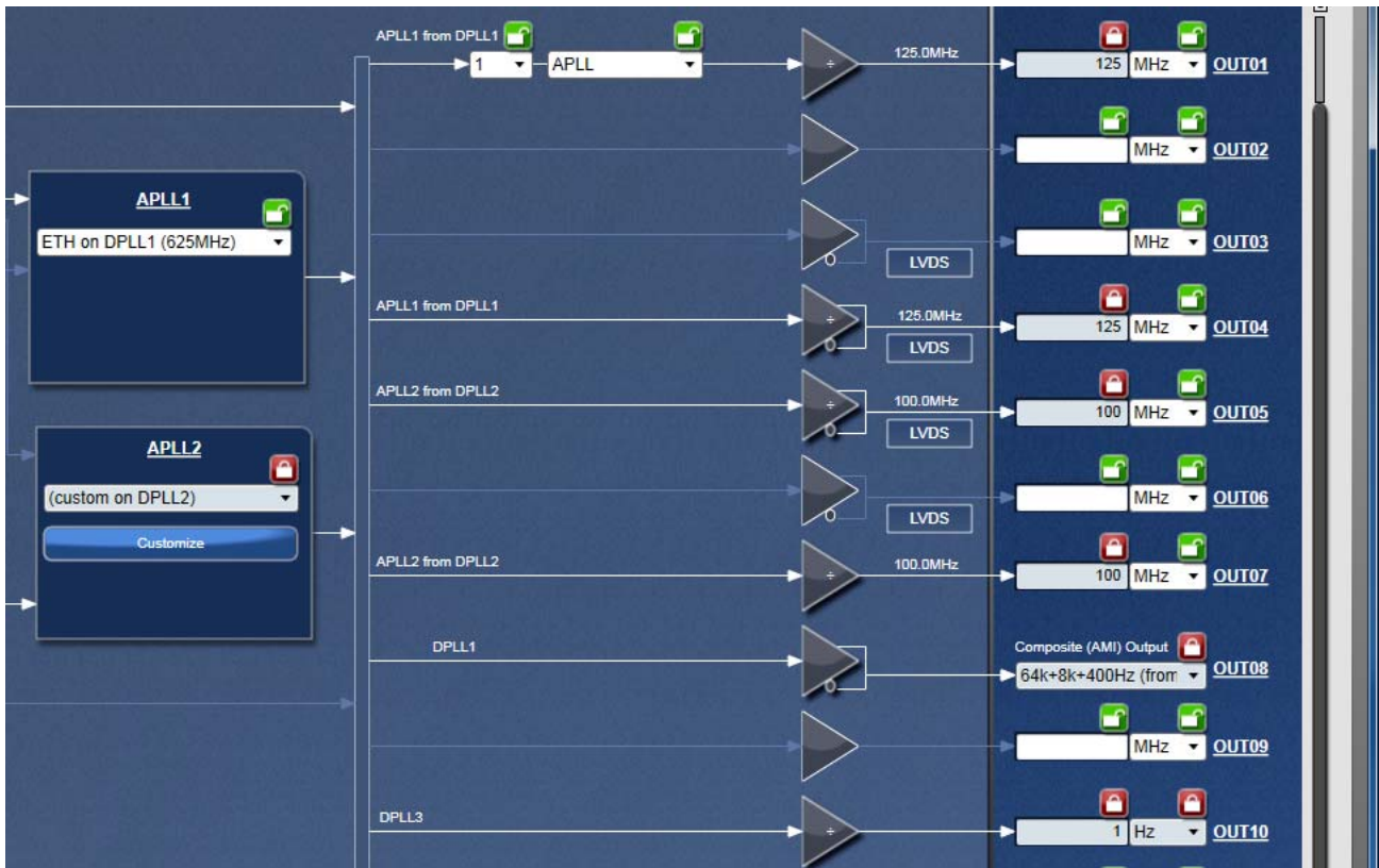
Figure 15. Output Frequencies Entered after APLL1/APLL2 Configured (example)
