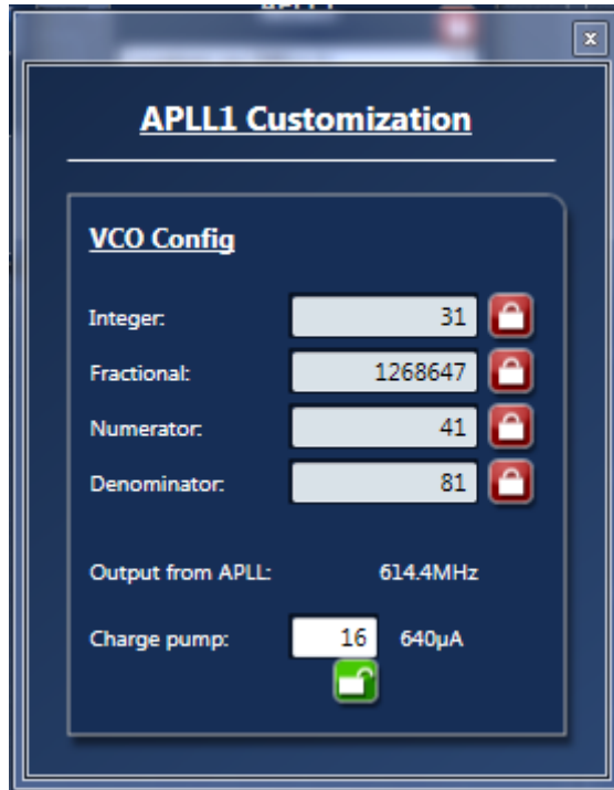
Figure 13. APLL1 Parameters for VCO = 614.4MHz
