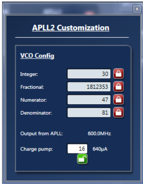
Figure 14. Configure APLL2 Parameters for VCO = 600.0MHz
