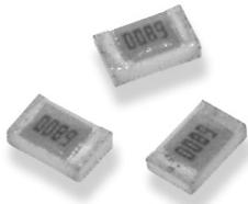
This tiny thin film chip is manufactured by sputtering pure metals onto a high purity alumina base. This process ensures the element remains stable in performance over a long life. The LT73 is equally suited to temperature compensation or thermal protection when incorporated within the appropriate electronics. This range of sensors are finished in a tough epoxy seal and are available on tape for high speed auto placement.
